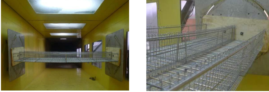
Fig. 7 Section model in wind tunnel
