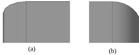
Fig. 3 Rounded corners of the train model (a) front corner elliptical rounding and (b) rear corner circular rounding
