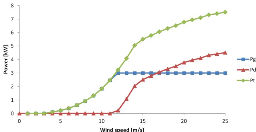
Fig. 8 Usable power ( $P_g$ ), power lost on dummy load ( $P_d$ ) and total power of the generator ( $P_t$ ) as functions of the incoming wind speed
