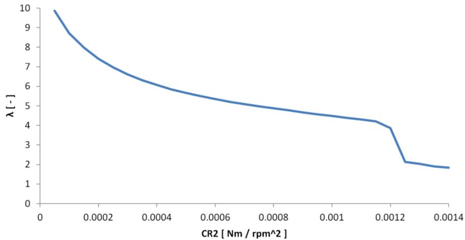
Fig. 6 Tip speed ratio as a function of the generator constant for region 2
