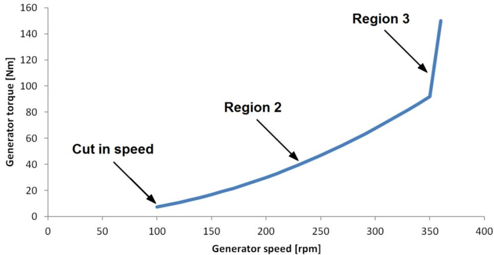
Fig. 4 Torque characteristic as a function of the generator rotor speed for a simple variable speed generator
