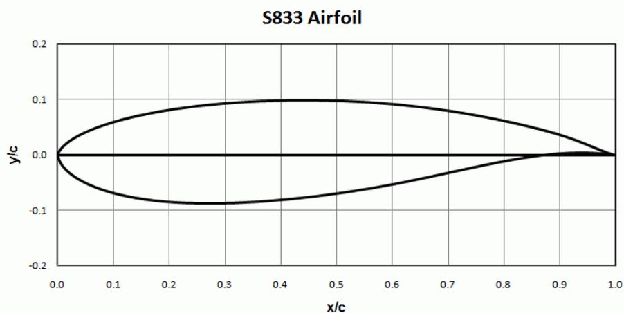
Fig. 3 S833 aerofoil proportions (used for the central portion of the blade) (Somers 2005)
