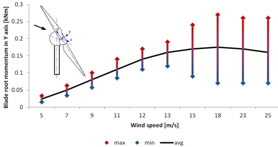
Fig. 13 Force momenta in blade root (min., max. and average) in Y-axis for the particular incoming wind speed values
