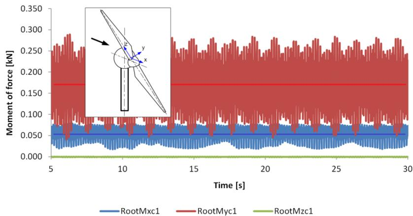
Fig. 10 Force momenta in the blade root recorded over simulation time
