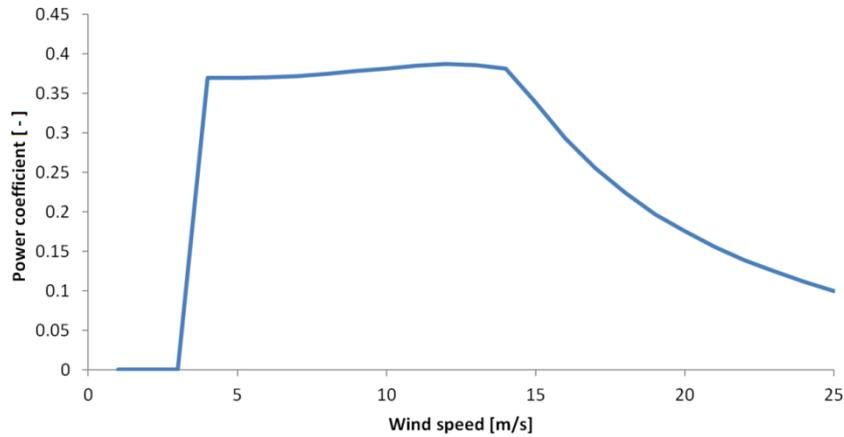
Fig. 9 Production coefficient (efficiency) of modelled STW as a function of the incoming wind speed
