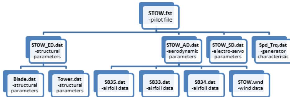
Fig. 2 FAST batch file structure used in the modelling procedure
