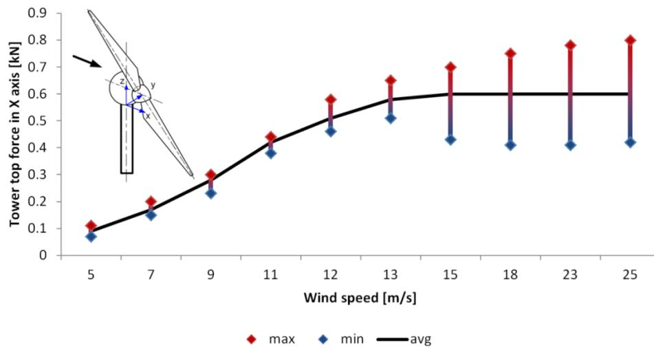
Fig. 14 Forces at the top of the tower (min., max. and average) in X-axis for the particular incoming wind speed values
