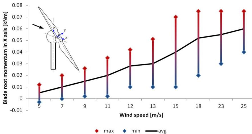
Fig. 12 Force momenta in the blade root (min., max. and average) in X-axis for the particular incoming wind speed values
