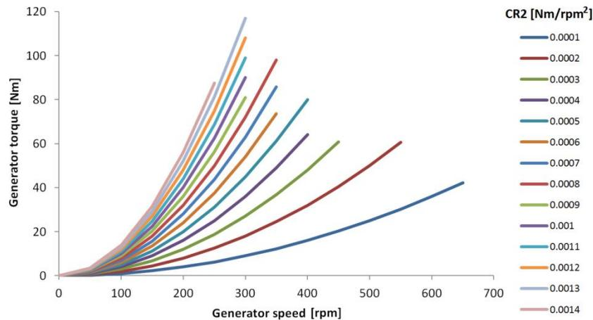
Fig. 5 Generator torques as functions of angular velocities for considered generator constants in region 2
