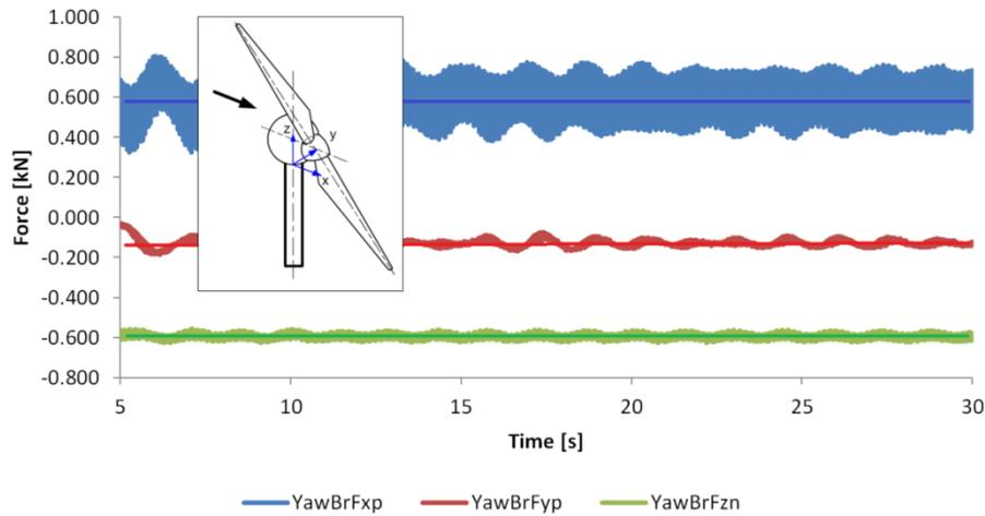
Fig. 11 Forces at the top of the tower recorded over simulation time
