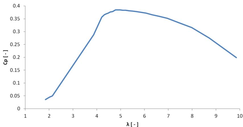
Fig. 7 Coefficient of power (efficiency) as a function of blade tip speed ratio
