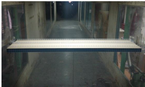
(a) Sectional rigid model and suspending system
