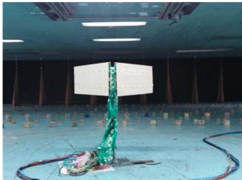
Fig. 8 Three-plate model in the wind tunnel
