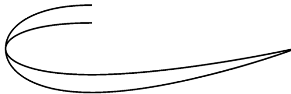
Fig. 2 The schematic of J-shaped airfoil of NACA0018 and NACA0030
