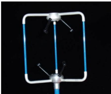
(a) 3D ultrasonic anemometer
