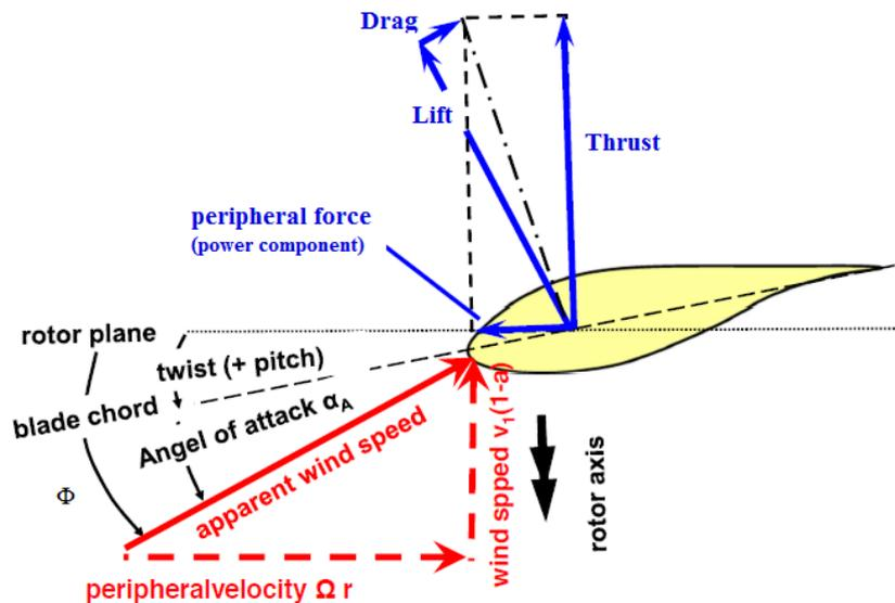
Fig. 1 Schematic of velocity and forces acting on HAWT blade element. Taken from Kühn (2013)
