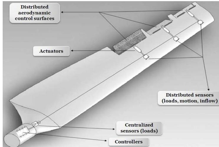
Fig. 5 Design view of a smart rotor blade. Taken from Barlas and Kuik (2010)
