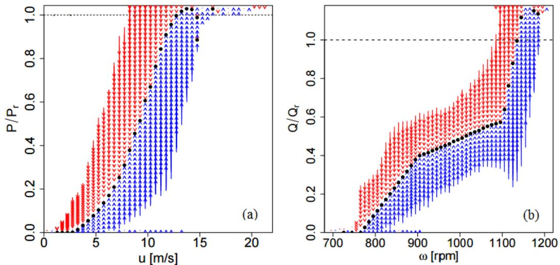
Fig. 3 Power output and rotor torque with drift function representing the local dynamics around stable fix points derived from wind turbine measurements. The stable fix points (black dots) are the points of attraction where drift function is zero. (a) Power output versus wind speed and (b) rotor torque versus angular speed. Power output and torque are normalized with their respective rated values. Taken from Wächter *et al.* (2012)
