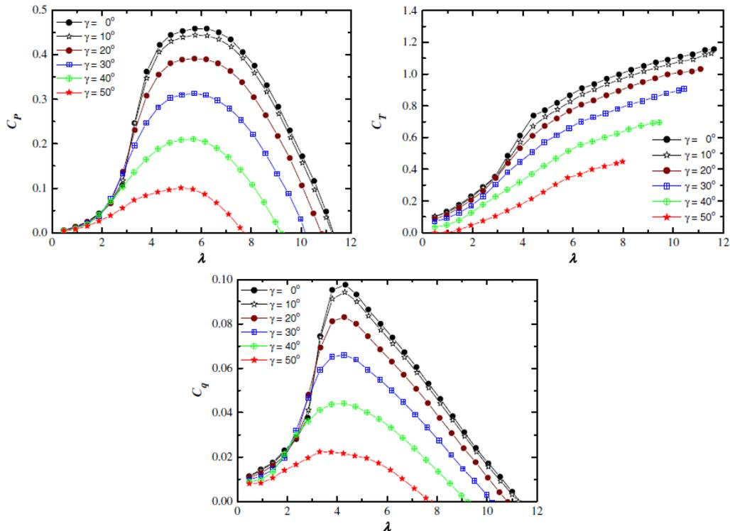
Fig. 3 Performance characteristics for a model turbine at different yaw angles. (a) Power coefficient and (b) thrust coefficient and (c) torque coefficient. Taken from Krogstad and Adaramola (2012)
