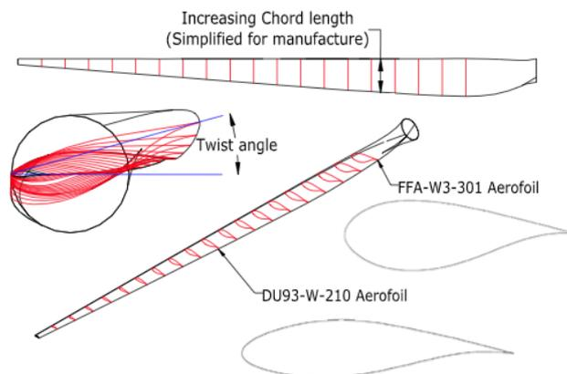
Fig. 2 HAWT blade with multiple airfoil profiles and shape distribution along the span. Taken from Schubel and Crossley (2012)
