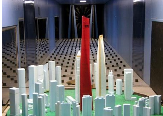
Fig. 4 Aerodynamic optimization by twisting
