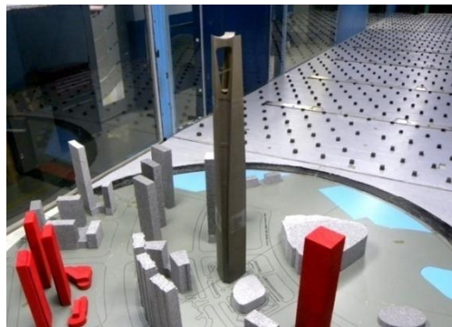
Fig. 5 Aerodynamic optimization by sculptured top
