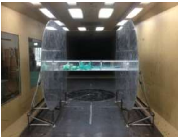
Fig. 3 View from upstream of the sectional model installed in the wind tunnel
