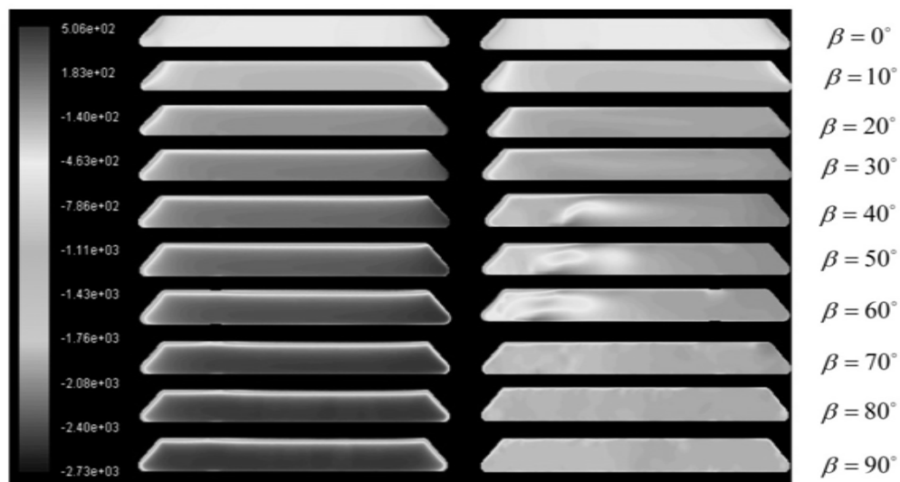
Fig. 8 Pressure distribution for the leeward (right) and windward (left) sides
