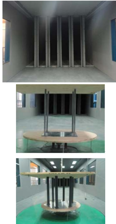
Fig. 5 Wind tunnel simulation of homogeneous turbulence and test models
