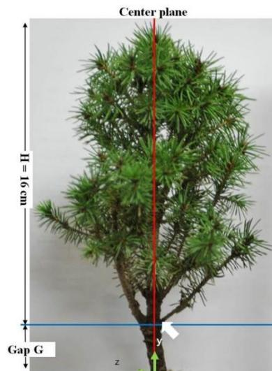
Fig. 3 A fir tree model tested in this study
