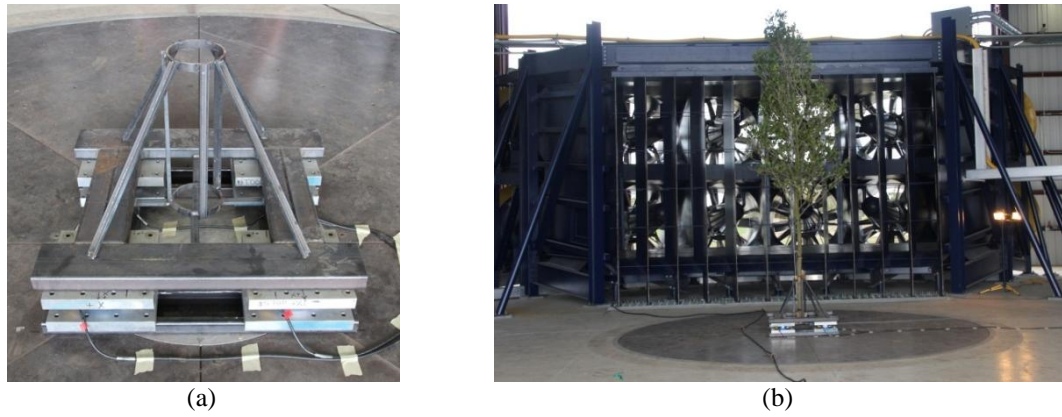
Fig. 6 Full-scale WoW testing (Phase 1): (a) steel frame mounted on load cells and (b) the overall test set in the test section
