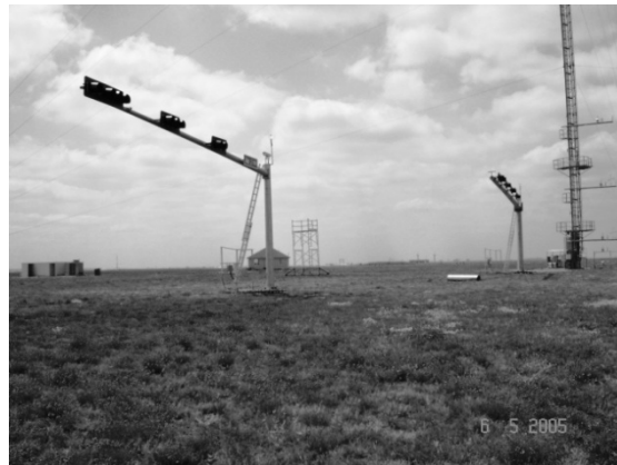
Fig. 3 The two cantilever traffic signal structures tested at Reese Technology Center
