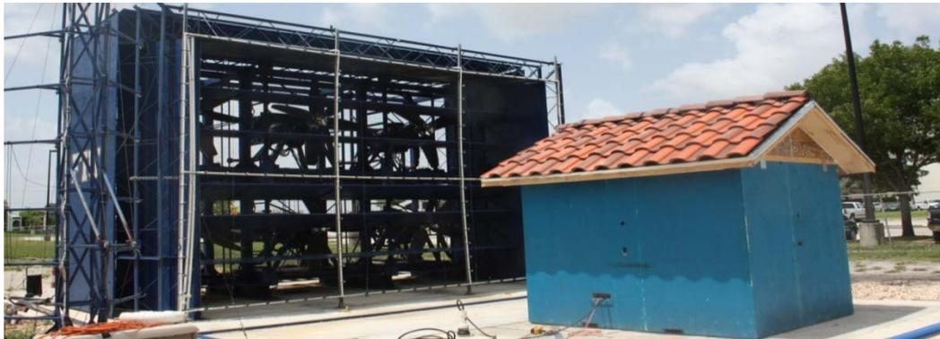
Fig. 2 Test specimen in front of Wall of Wind at 0° AoA
