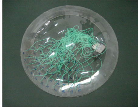
Fig. 3 Testing points on dome model
