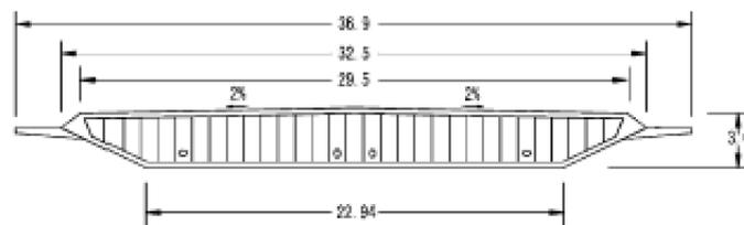
Fig. 4 Cross section of deck of Jiang Yin Bridge (Unit: m)
