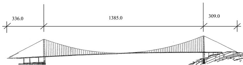
Fig. 3 Elevation of Jiang Yin Bridge (Unit: m)
