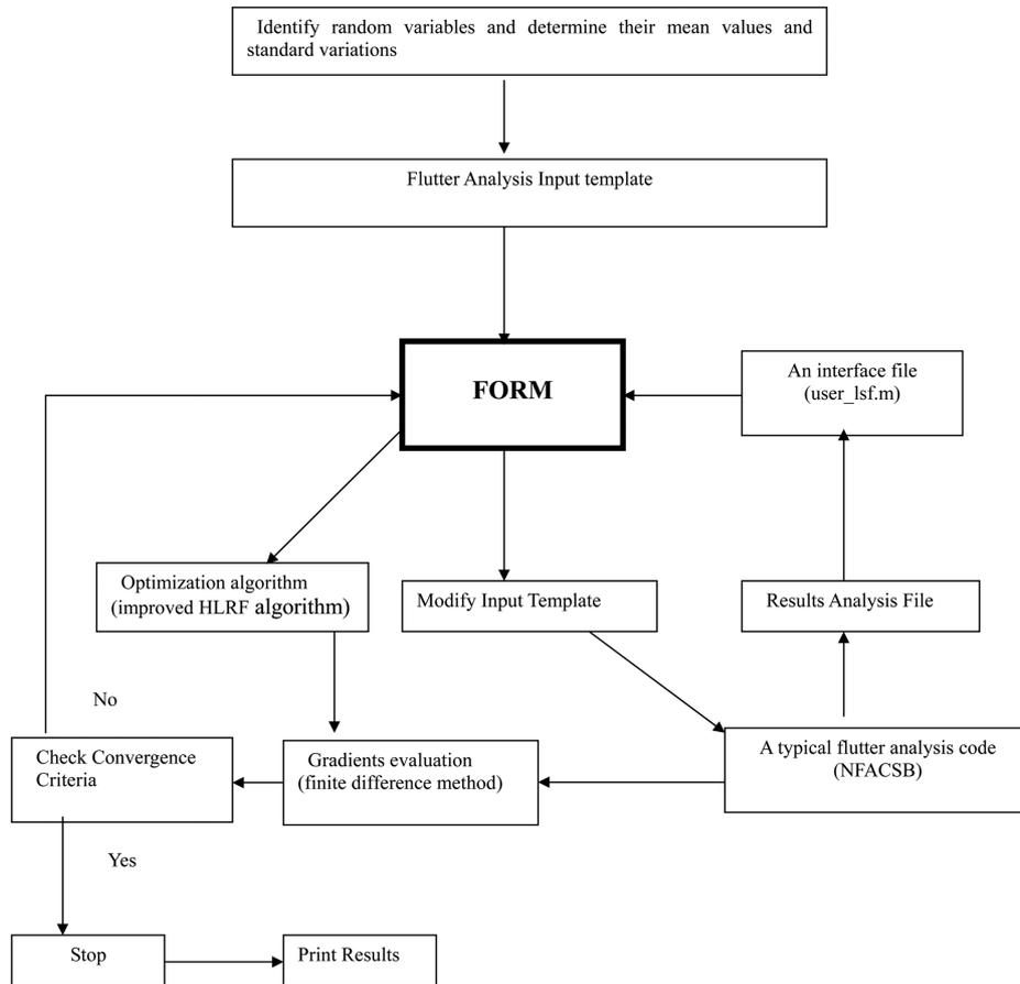
Fig. 2 Architecture of the FORM based flutter reliability analysis method in FREASB
