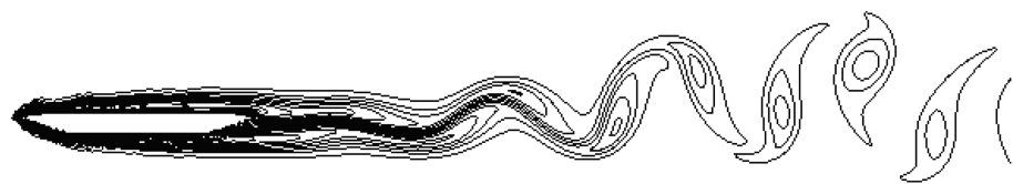
Fig. 9 Contour plot of vorticity in flow by PSE (Sutong Bridge)
