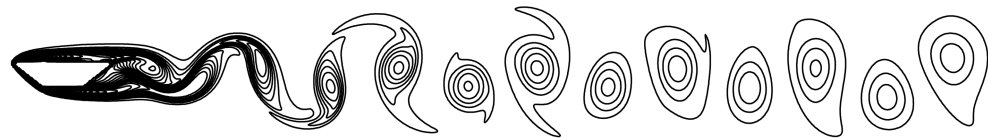
Fig. 5 Contour plot of vorticity in flow by PSE (Great Belt East Bridge)
