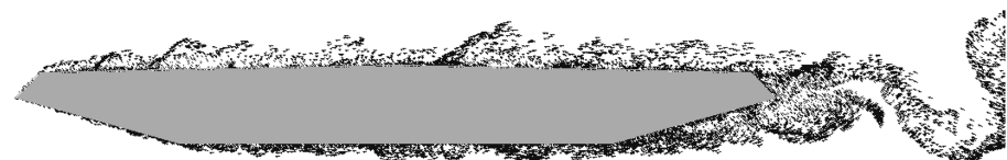
Fig. 10 Instant flow patterns around the deck section (Sutong Bridge)
