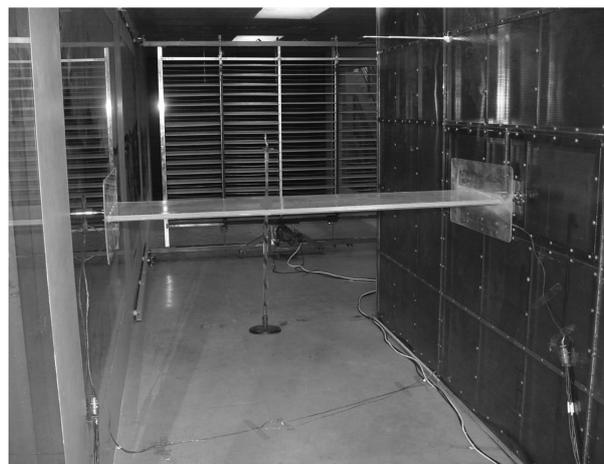
Fig. 7 The thin plate section model in the wind tunnel
