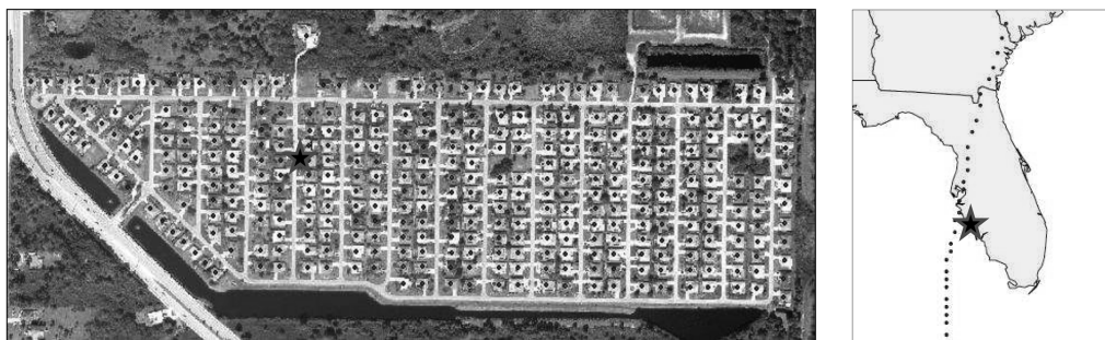
Fig. 7 Study area of a residential development of 358 houses in Sarasota County, Florida (left; the dots represent the centers of the houses) and simulated storm track of Hurricane Charley of 2004 (right). The star (in both panels) represents the recording location of the wind time history during the passage of the simulated storm
