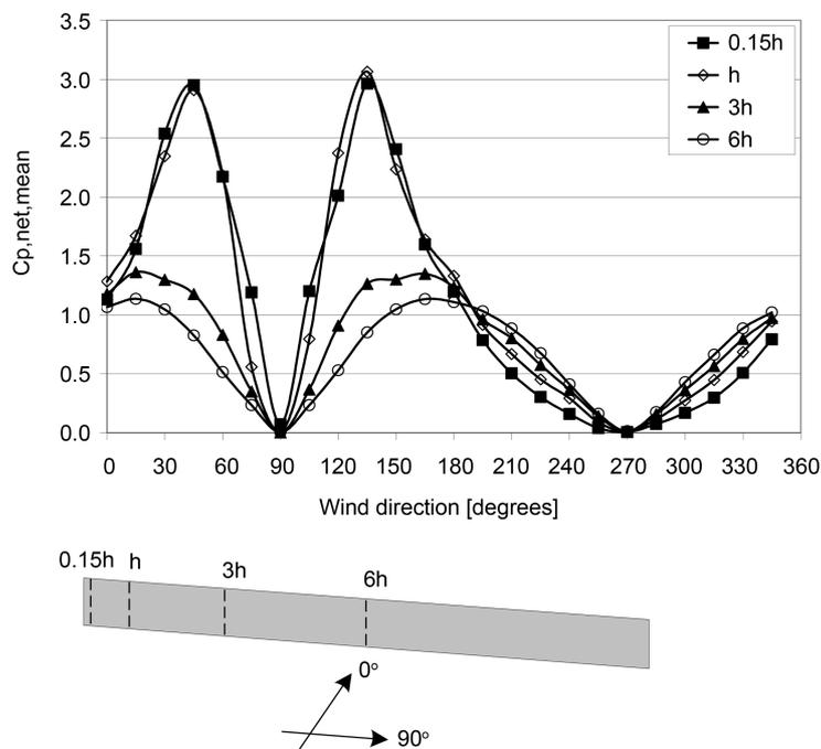
Fig. 5 Mean net pressure coefficients for configuration 2, vertical wall of 8 m without T-top
