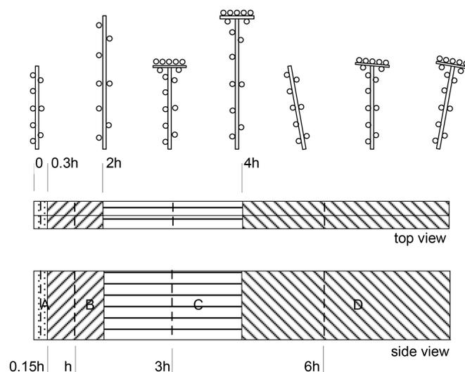
Fig. 4 Positions of pressure taps (top); position of taps in relation to zones of EN 1991-1-4 (bottom)
