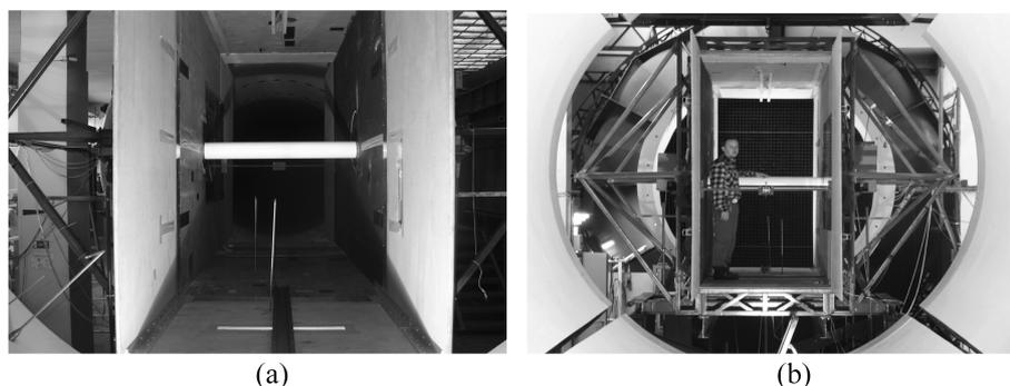
Fig. 2 VKI low speed wind tunnel with rectangular insert equipped with strain gauge balances and one of the circular cylinder: (a) front view; (b) back view
