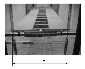
Fig. 2 Bridge sectional model suspended by a custom-designed rig-spring mechanism
