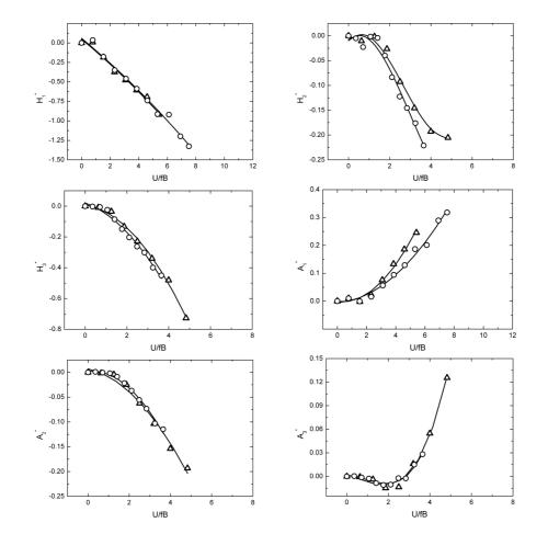
Fig. 7 Flutter derivatives of model with 35% gap-width  $\Delta$ : frequency ratio =1.2 o: frequency ratio =2.2
