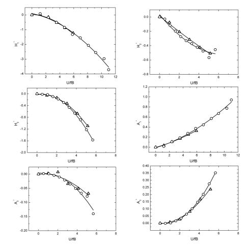
Fig. 5 Flutter derivatives of model with a zero gap-width  $\Delta$ : frequency ratio =1.2 o: frequency ratio =2.2
