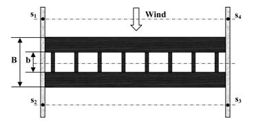
Fig. 4 Top view of model-rig system and the layout of laser sensors (s<sub>1</sub>, s<sub>2</sub>, s<sub>3</sub> and s<sub>4</sub>)
