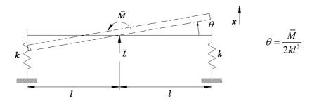
$\overline{M}$ : mean of pitching moment  $\overline{L}$ : mean of lift force  $\theta$ : additional angle of wind incidence
