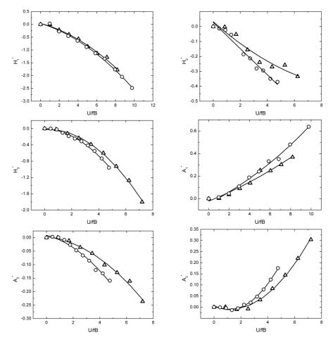
Fig. 6 Flutter derivatives of model with 16% gap-width  $\Delta$ : frequency ratio =1.2 o: frequency ratio =2.2
