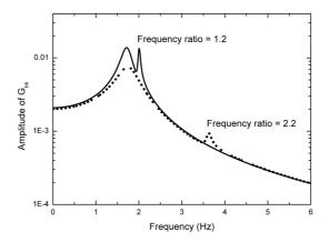
Fig. 1 Typical Frequency Response Function (FRF) of the 2DOF model-rig bridge dynamic system
