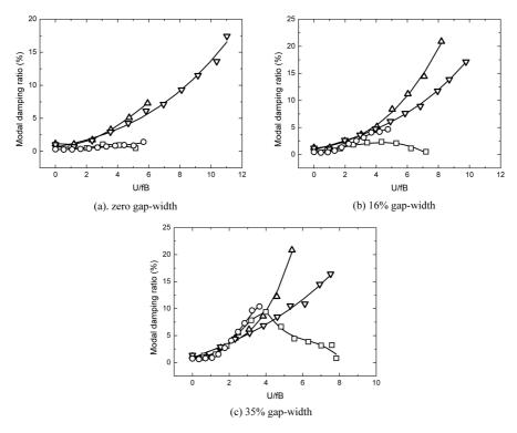
Fig. 9 Modal damping ratios of configurations with different gap-widths
