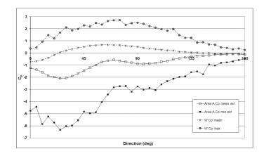
Fig. 4 Peak and mean pressure coefficients on areas A and W as a function of wind angle
