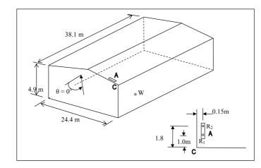
Fig. 3 Full scale dimensions and pressure tap locations on the NIST building also showing roof corner region C (not to scale)
