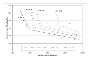
Fig. 8 S-N curve for corrugated cladding fastened without cyclone washers
