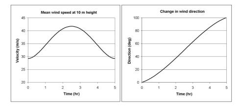
Fig. 2 Variation of mean wind speed and direction over time (Jancauskas, et al. 1994)
