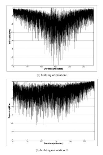
Fig. 6 Net pressures for varying wind angle and mean wind speed over time
