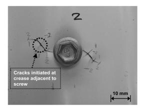
Fig. 11 Cracking of cladding at screw fixing
