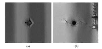
Fig. 12 Cracking patterns following L-H-L tests of cladding that (a) failed and (b) passed but had a 15% reduction in load per cycle
