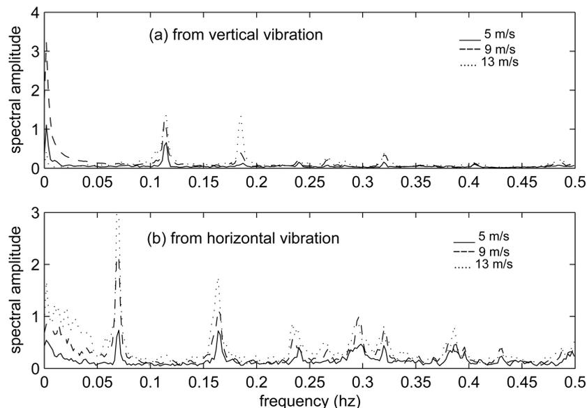
Fig. 6 Auto-power spectrum of vibration at different wind speeds
