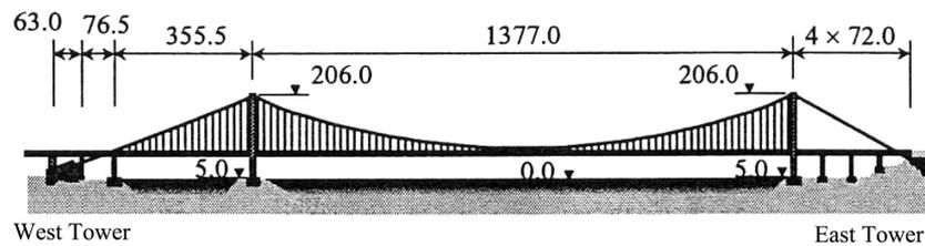
Fig. 1 Elevation of the suspension bridge (dimensions in metre)
