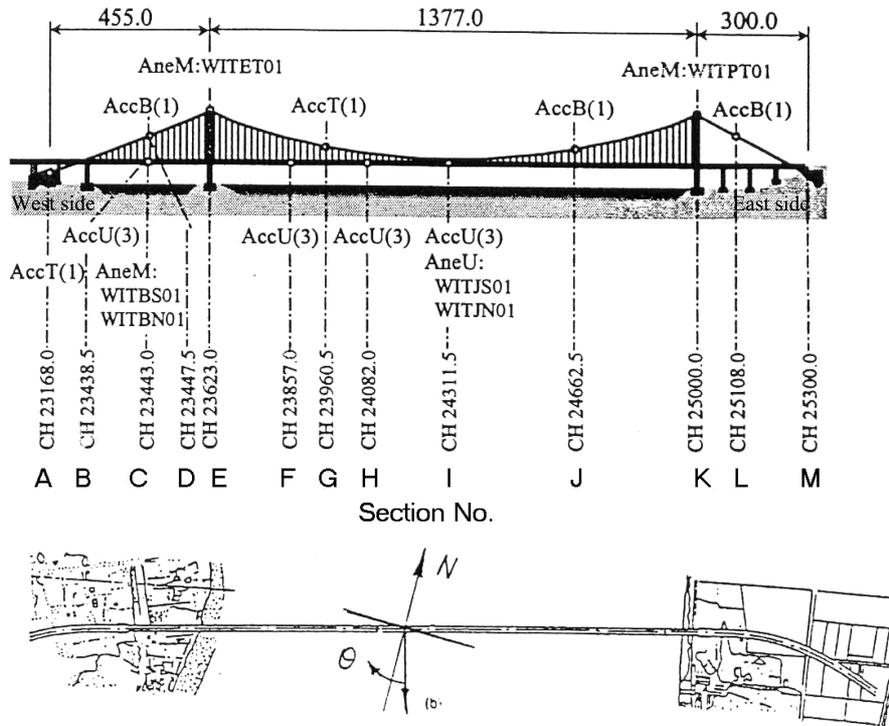
Fig. 4 Location of instruments (dimensions in metre)
