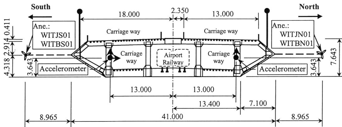
Fig. 2 Cross-section of bridge deck and sensor locations (dimensions in metre)
