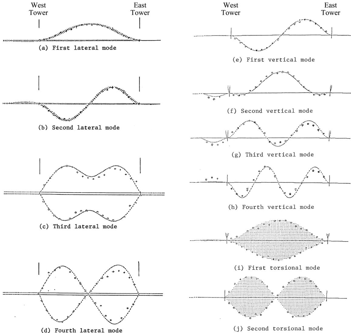
Fig. 3 Vibration mode shapes (+, o measurement points)
