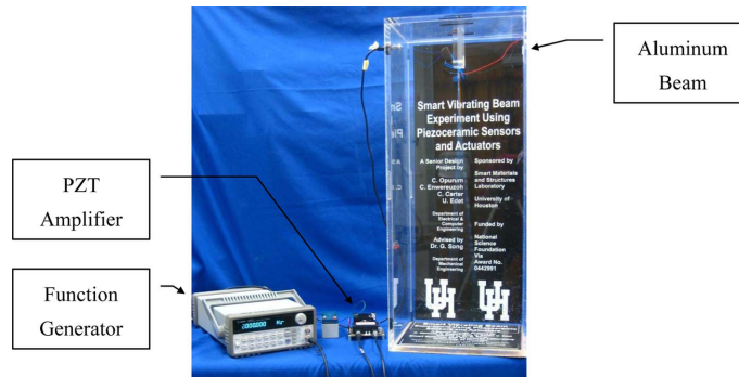
Fig. 11 Vibration control of an aluminum beam experiment setup
