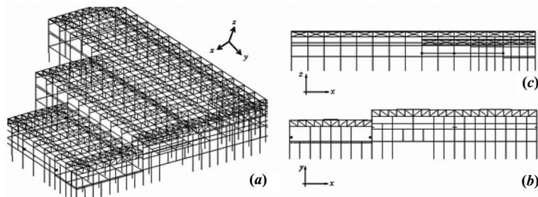
Fig. 12 3D view (a) front view (b) and lateral view (c) of the FE model
