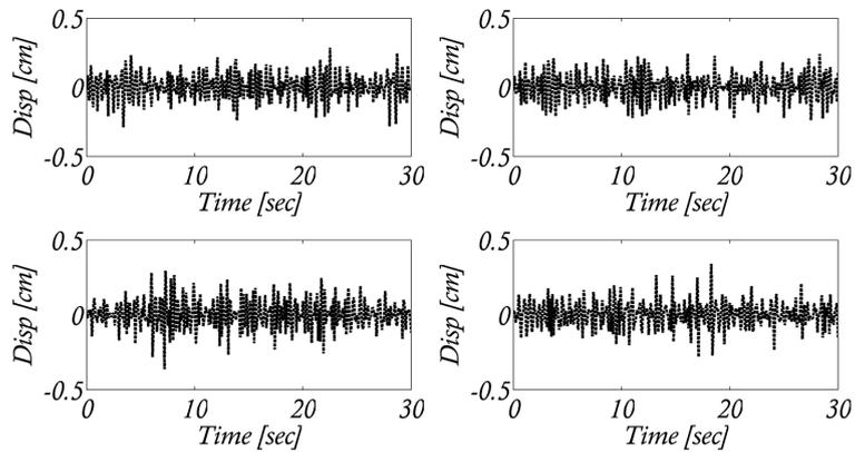
Fig. 7 GPS recorded displacements time histories along the  $X$  (left side plots) and  $Y$  axes (right side plots). Top: GPS “ $c$ ” displacements. Bottom: GPS “ $b$ ” displacements
