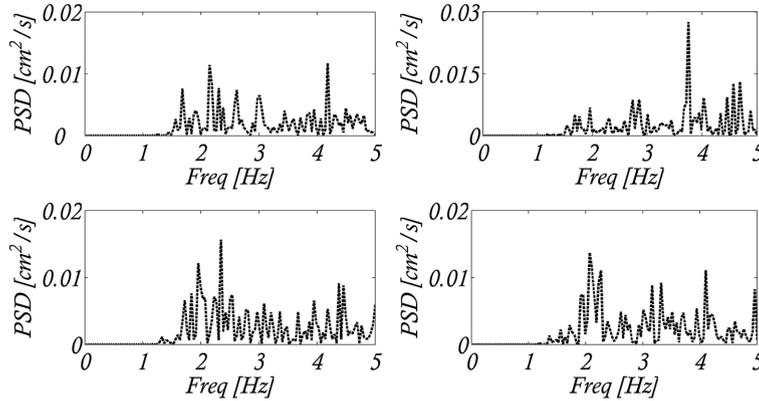
Fig. 9 PSD functions from the GPS measurements along  $X$  (left side plots) and  $Y$  axes (right side plots), Top: PSD of the GPS unit “ $c$ ”. Bottom: PSD of the GPS unit “ $b$ ”
