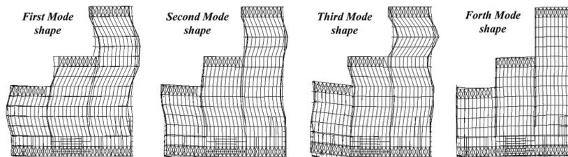
Fig. 14 Numerical mode shapes referring to the final constraints condition (case 2)
