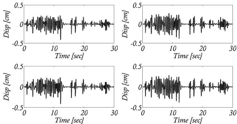
Fig. 8 Accelerometers calculated displacements time histories along the  $X$  (left side plots) and  $Y$  axes (right side plots). Top: Acc. “ $c$ ” displacements. Bottom: Acc. “ $b$ ” displacements
