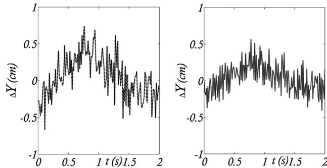
Fig. 15 Test under the deceleration force induced by the bridge-crane: experimental results from GPS receiver “c” data (left), numerical results (right)
