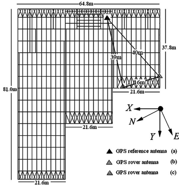
Fig. 4 GPS configuration in the  $N-E$  and  $X-Y$  plane.  $\alpha$  is the angle between axes  $X$  and  $N$
