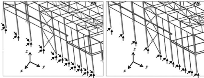
Fig. 13 Details on the constrains of the columns supporting the bridge-crane: fixed supports condition (on the left - case 1); final constraints condition (on the right - case 2)
