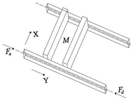
Fig. 16 Scheme of bridge-crane forces during vibration tests
