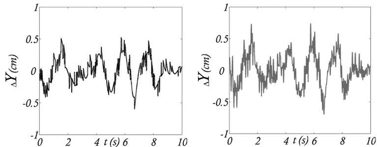
Fig. 17 Structural Displacement of the deceleration-acceleration force: experimental results from GPS receiver “c” data (left), numerical results (right)
