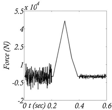
Fig. 18 Calculated FE model input impact force
