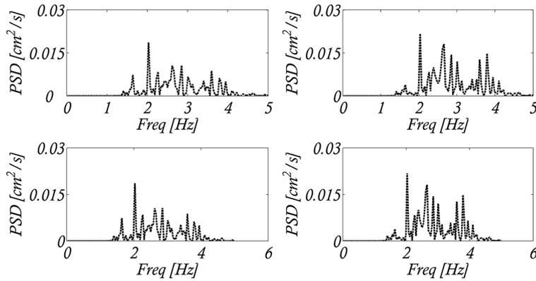
Fig. 10 PSD functions from the accelerometers calculated displacements along  $X$  (left side plots) and  $Y$  axes (right side plots), Top: PSD of Acc. “ $c$ ” data, Bottom: PSD of Acc. “ $b$ ” data
