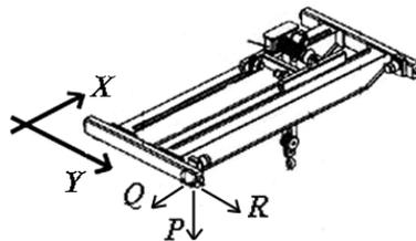
Fig. 5 Bridge-crane reaction forces in the  $X-Y$  plane
