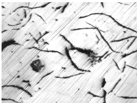
Graphite flakes in gray cast iron
