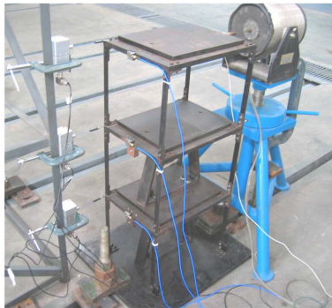
(a) A 3-Story test building model
