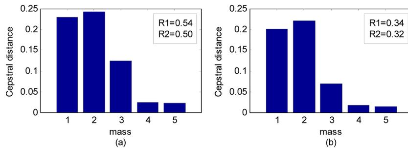
Fig. 4 5-DOF system with 24% stiffness reduction in the 2<sup>nd</sup> storey (data length = 9000, SNR = 10): (a) without ACW and (b) with ACW
