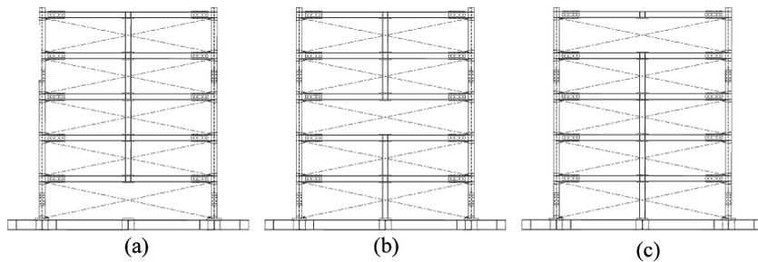
Fig. 11 Damage case: removing central column on the (a) first, (b) third and (c) fifth floor
