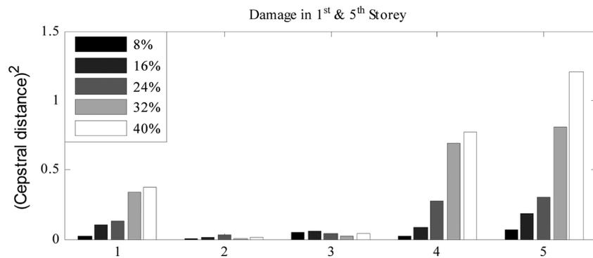
Fig. 9 Cepstral distance for the multiple damage case (data length = 9000)
