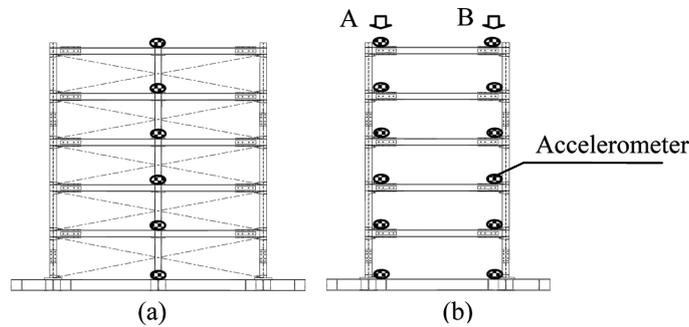
Fig. 10 Tested building model: (a) long-side and (b) short-side
