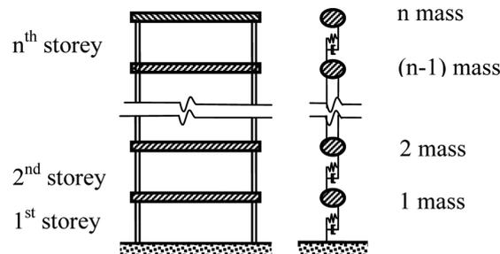
Fig. 2 Simplified structural model
