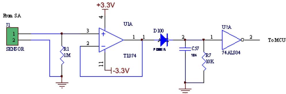
Fig. 5 Impact detection circuit
