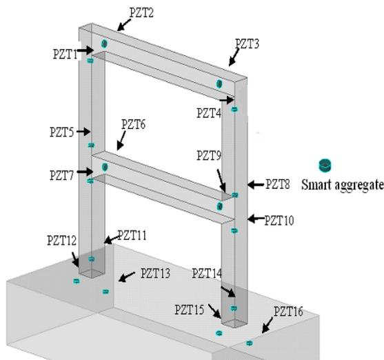
Fig. 14 Two-story concrete frame with embedded smart aggregates
