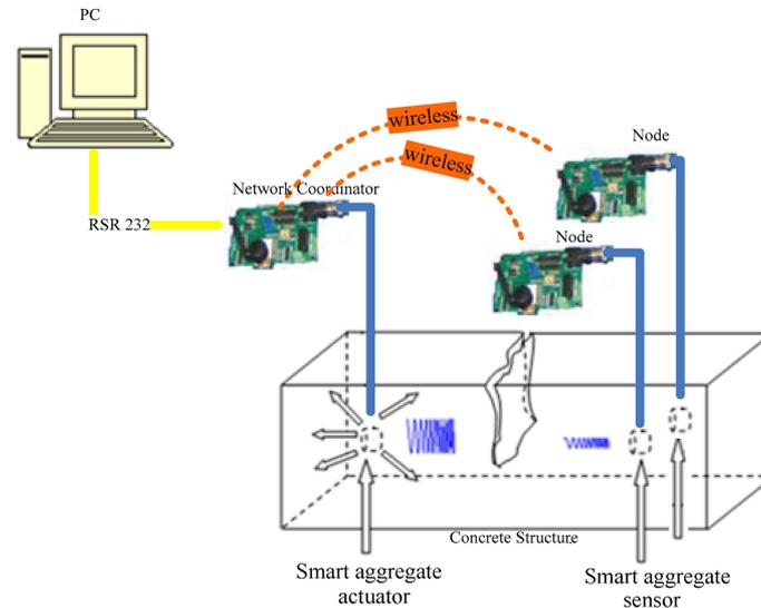
Fig. 3 Block diagram of piezoelectric-based active sensing system
