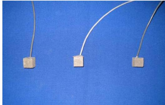
Fig. 1 Photos of piezoceramic-based smart aggregate
