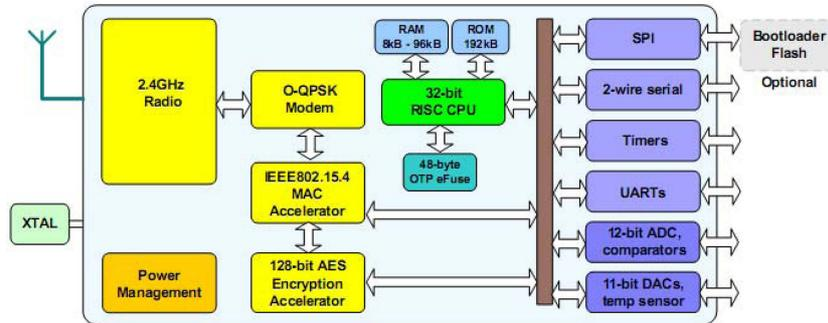
Fig. 8 System block diagram for JN5139
