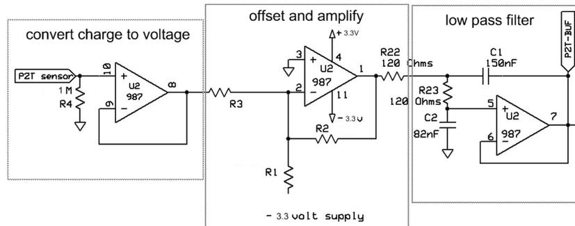
Fig. 6 Signal conditioning circuit
