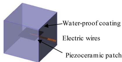
Fig. 2 Illustration of a smart aggregate
