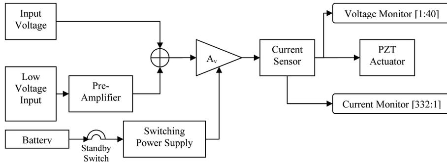
Fig. 7 Power amplifier for the PZT actuation
