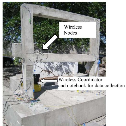
Fig. 15 Photo of the two-story concrete frame
