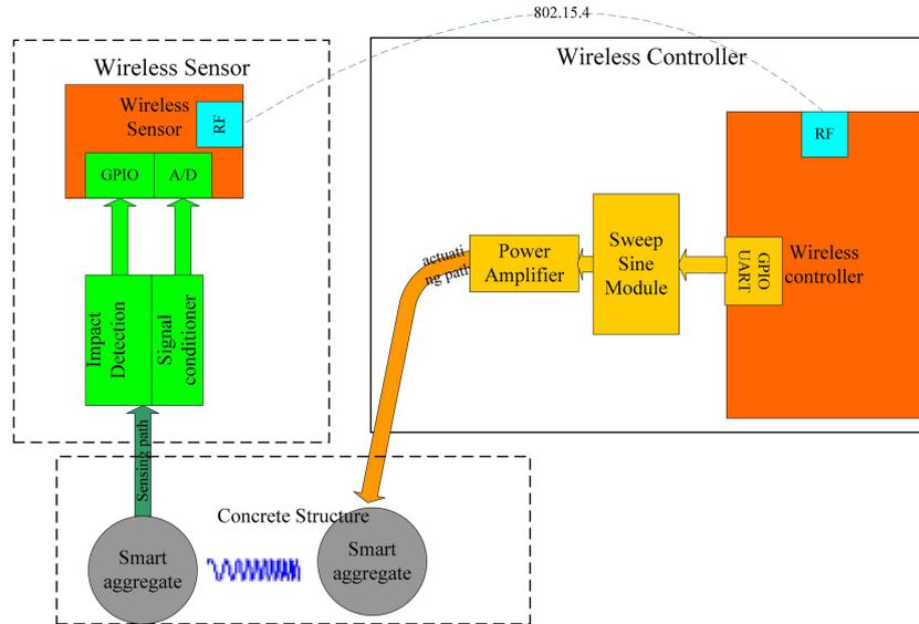
Fig. 4 The wireless system architecture
