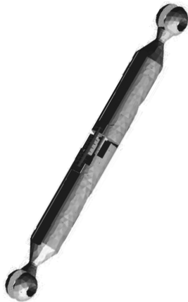
Fig. 21 Model of adaptronic strut by CAD data
