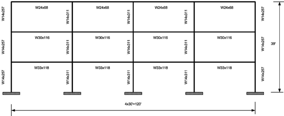
Fig. 3 Four-bay 3-story rigidly connected frame (Model-3)
