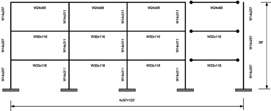
Fig. 2 Four-bay 3-story simply connected frame (Model-2), (Ohtori, *et al.* 2004)
