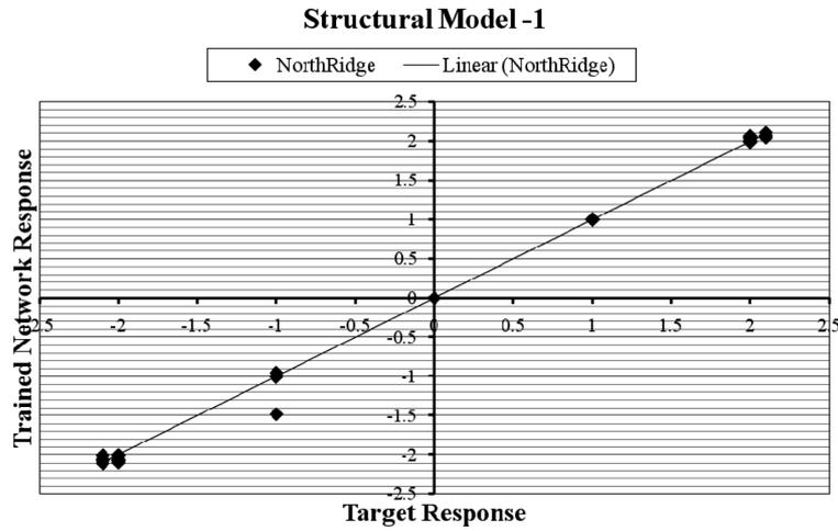
Fig. 14 Testing data performance for NorthRidge earthquake Model-1
