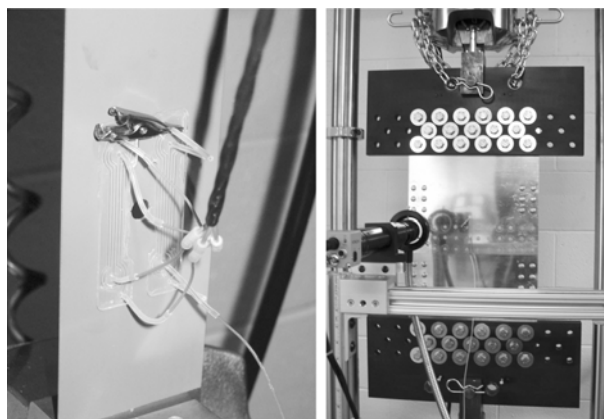
Fig. 6 CVM sensors monitoring crack growth on aluminum test specimens
