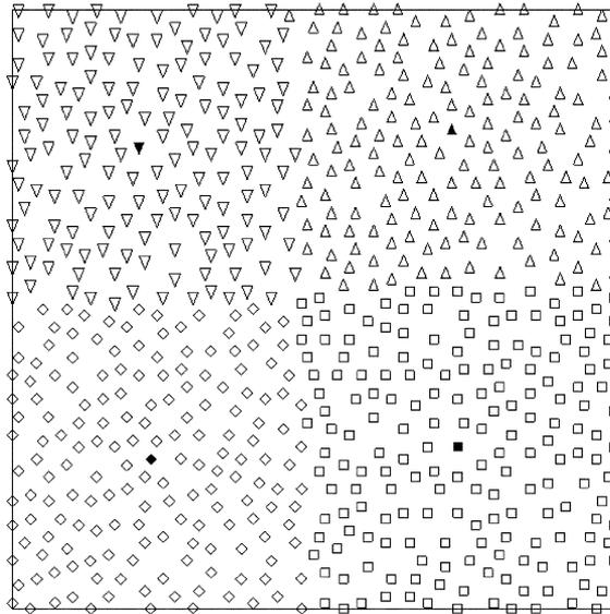
Fig. 2 Four clusters  $A$  (upper triangle),  $B$  (square),  $C$  (diamond),  $D$  (low triangle) and a master sensor (solid) for each cluster are assigned after 8 iterations
