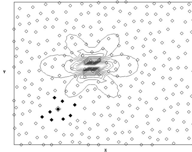
Fig. 6 True damage location is distinguished by von Mises stress contours generated by ABAQUS FE simulation. Initial stage of damage tracking process: one of the mater sensors (double diamond) activates 8 neighboring sensors (solid diamond). Activated sensors communicate each other to find the biggest gradient of measured strain value
