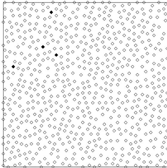
Fig. 1 Four master sensors are randomly selected out of total 679 sensors (hollow diamond). The minimum distance between neighboring sensors is limited to 3 m
