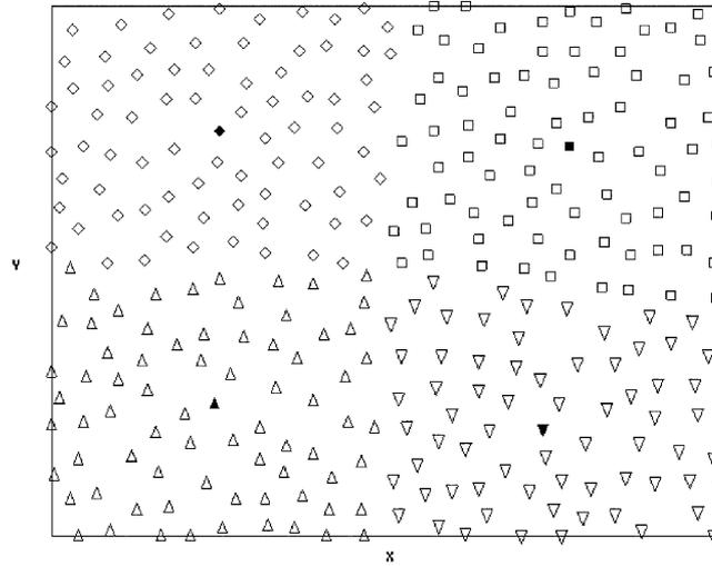
Fig. 5 Four clusters *A* (upper triangle), *B* (square), *C* (diamond), *D* (low triangle) and four master sensors (solid) are assigned out of total 300 sensors over the plate. The minimum distance between neighboring sensors is limited to 2.5 m
