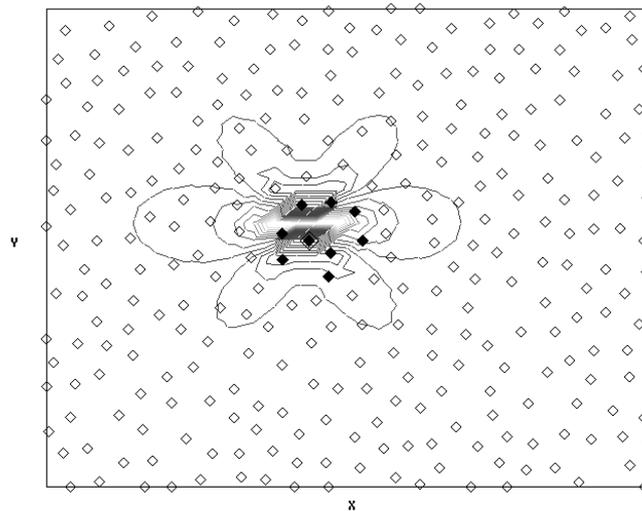
Fig. 8 After five iterations of damage tracking process: mater sensor (double diamond) does not activate neighboring sensors (solid diamond) any longer because no more gradient can be found
