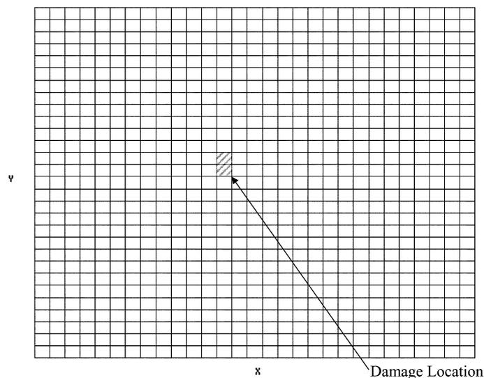
Fig. 4 ABAQUS FE model of a plate (25 m×20 m×0.5 m) having two stiffness-reduced elements out of total 900 elements to simulate the stress condition of a damaged structure
