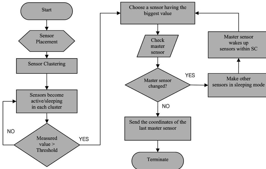
Fig. 3 Overall flow chart for decentralized damage detection procedure
