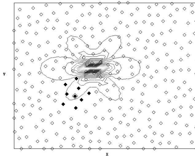
Fig. 7 True damage location is distinguished by von Mises stress contours generated by ABAQUS FE simulation. Initial stage of damage tracking process: one of the mater sensors (double diamond) activates 8 neighboring sensors (solid diamond). Activated sensors communicate each other to find the biggest gradient of measured strain value
