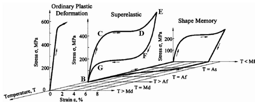
Fig. 1 3D stress-strain-temperature ( $\sigma$ - $\varepsilon$ - $T$ ) diagram of SMA showing SME in martensite state, PE during austenite/martensite phase transformation and elastic-plastic behaviour of austenite at higher temperature (reprinted from DesRoches, *et al.* 2004 with permission)
