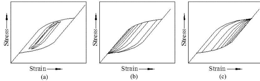
Fig. 3 1D-Superelastic model of SMA at constant temperature where the stress-strain curves are drawn after a complete transformation path followed by (a) PL and PU, (b) PL and CU, and (c) CL and PU (reprinted from Auricchio, *et al.* 1997 with permission)
