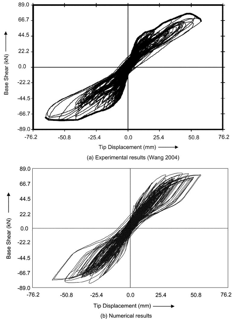
Fig. 5 Load versus tip-displacement for SMA-steel coupled reinforced concrete bridge pier under earthquake type loading
