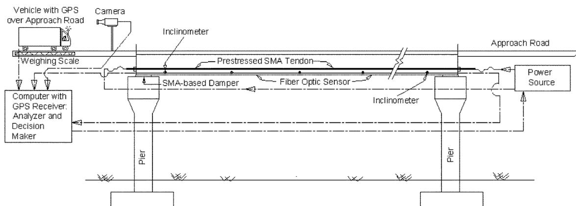
Fig. 8 Highly instrumented SMA-based smart RC bridge
