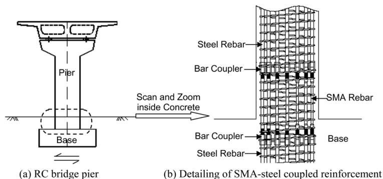
Fig. 4 RC bridge pier reinforced with coupled SMA-steel rebar
