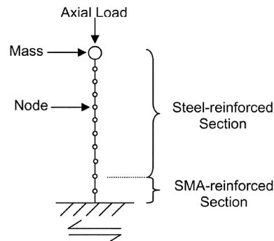
Fig. 6 Finite element model for SMA reinforced concrete column
