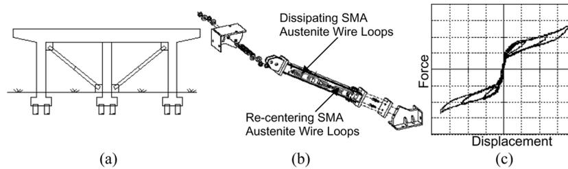
Fig. 10 (a) Retrofitting of highway RC bridges with SMA-based supplemental re-centering bracing, (b) arrangement of the SMA wires inside the device and (c) typical cyclic force-displacement behaviour (reprinted from Cardone *et al.* 2004 with permission)
