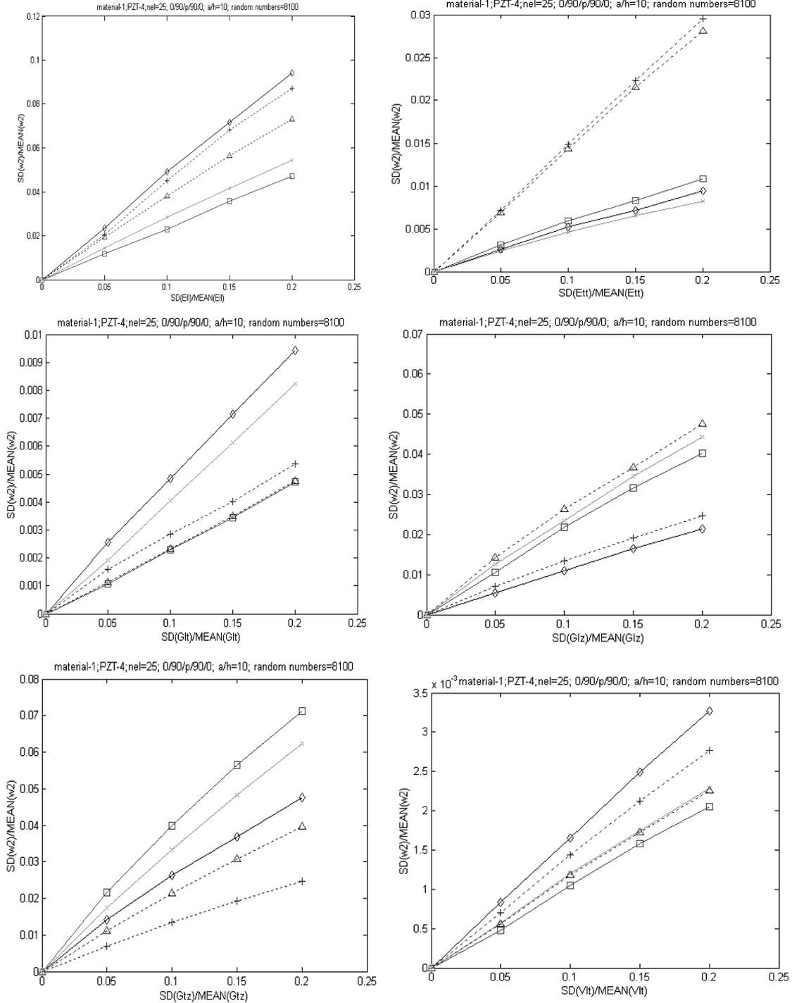
Fig. 6 Influence of SD of basic material properties on SD of the first five natural frequencies, for [0/90/p/90/0] laminate (a) only  $E_{II}$  varying, (b) only  $E_{II}$  varying, (c) only  $G_{II}$  varying, (d) only  $G_{Iz}$  varying, (e) only  $G_{Iz}$  varying, (f) only  $\nu_{II}$  varying, Key: Same as in Fig. 4.
