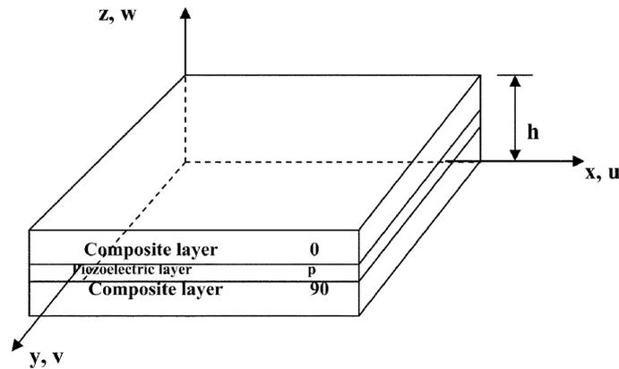
Fig. 1 Geometry of the laminated composite plate with piezoelectric layer
