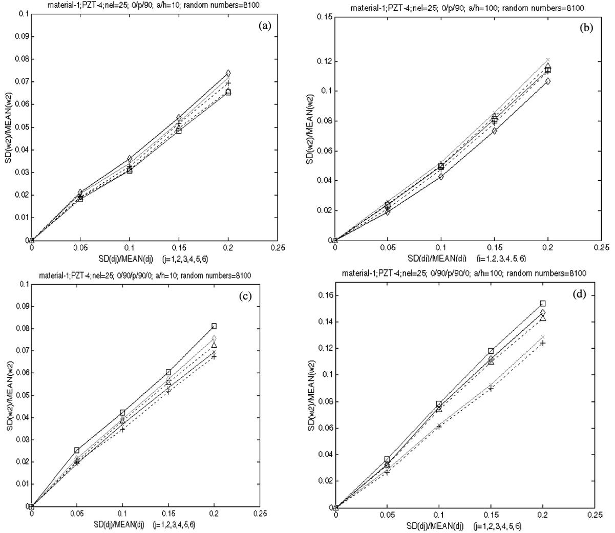
Fig. 4 The effect of varying all material properties simultaneously on  $\sigma\omega^2/\mu\omega^2$  of the first five mean frequencies of vibration. (a)  $a/h = 10$  and  $[0/p/90]$ , (b)  $a/h = 100$  and  $[0/p/90]$ , (c)  $a/h = 10$  and  $[0/90/p/90/0]$ , (d)  $a/h = 100$  and  $[0/90/p/90/0]$ . Key:  $\diamond$ : first mode,  $+$ : second mode,  $\square$ : third mode and  $\Delta$ : fifth mode
