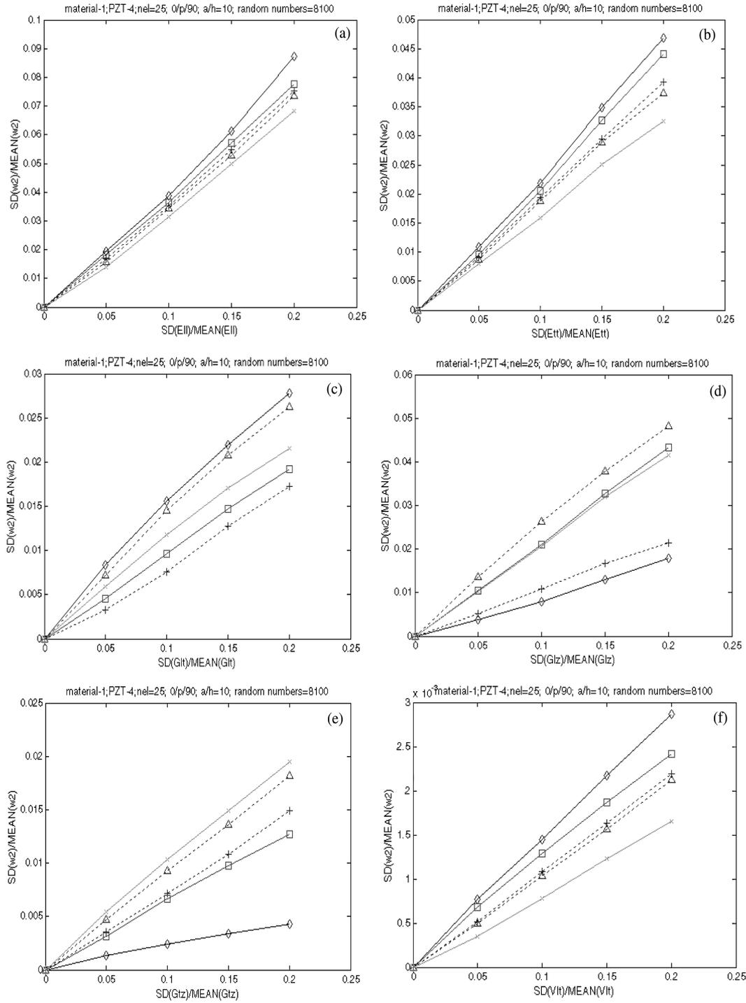
Fig. 5 Influence of the SD of basic material properties on the SD of the first five natural frequencies, for [0/p/90] laminate. (a) only  $E_{II}$  varying, (b) only  $E_{II}$  varying, (c) only  $G_{II}$  varying, (d) only  $G_{Iz}$  varying, (e) only  $G_{Iz}$  varying, (f) only  $\nu_{II}$  varying, Key: Same as in Fig. 4.
