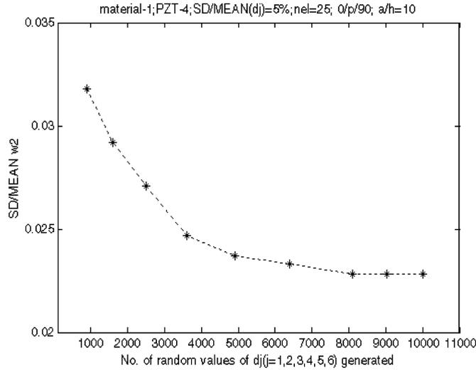
Fig. 2 Convergence study for random numbers to be generated for random variables with material properties varying simultaneously (dj)
