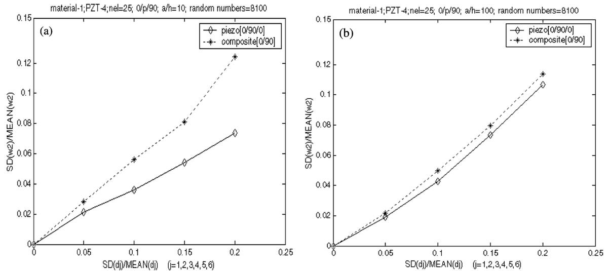
Fig. 3 Influence of SD of basic material properties on the SD of the fundamental frequency with all basic material properties changing at a time
