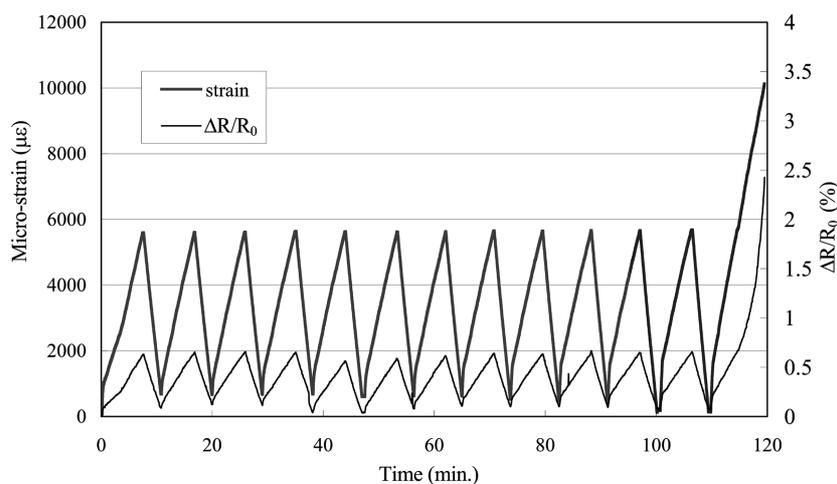
Fig. 3 Cyclic tension result of epoxy resin-impregnated C1 carbon tows
