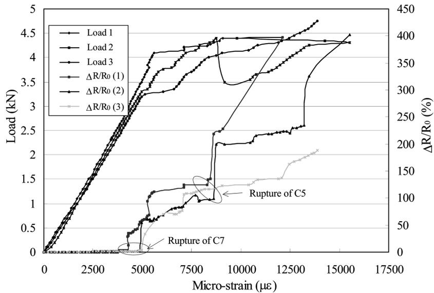
Fig. 8 Experimental results of specimens 1-3 with C1, C5 and C7 in a ratio of 3:1:1
