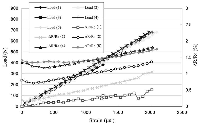
Fig. 4 Cyclic tension result of the C1C7 HCFRP sensor for the first five loading cycles before the micro-ruptures of carbon tows
