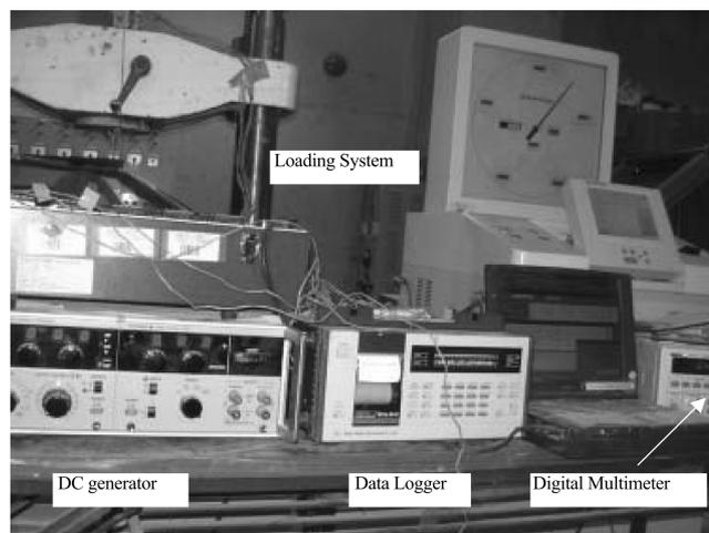
Fig. 2 Schematic illustration of experimental system
