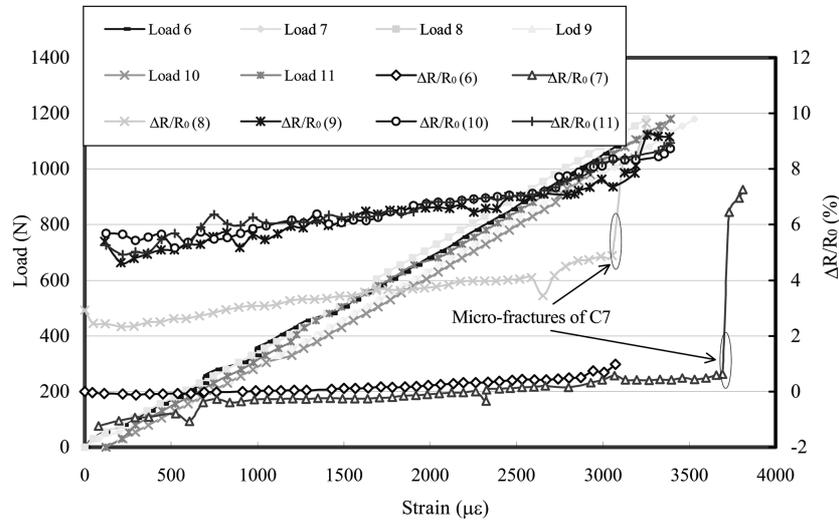
Fig. 5 Cyclic tension result of the C1C7 HCFRP sensor for the 6th-11th loading cycles around the micro-fractures of carbon tows
