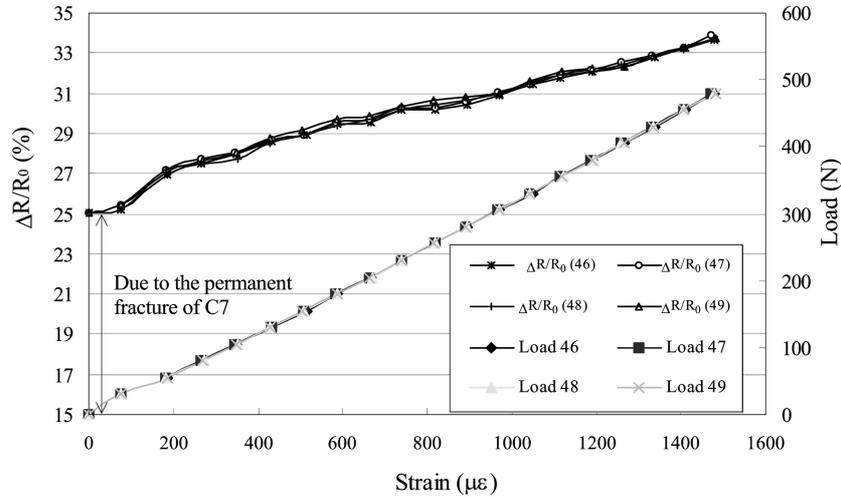
Fig. 6 Cyclic tension result of the C1C7 HCFRP sensor for the 46th-49th loading cycles after the micro-fractures of carbon tows
