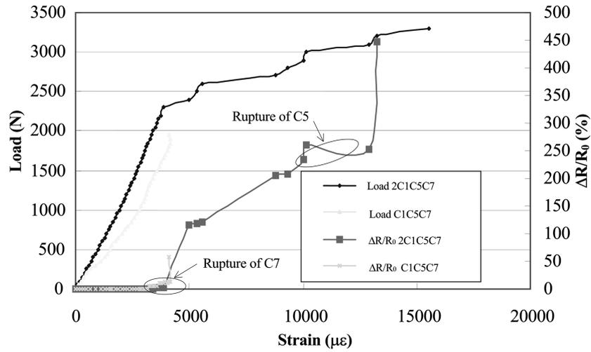
Fig. 7 Volume fractions of HS carbon tows on the electrical and mechanical behaviors of HCFRP sensors with three types of carbon tows
