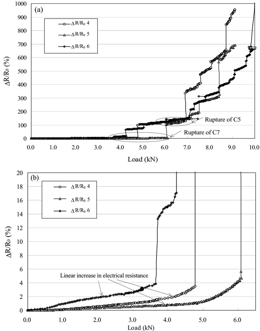
Fig. 10 Evolutions of  $\Delta R/R_0$  as a function of load for specimens 4-6 with C1, C5 and C7 in a ratio of 1:1:1 adhesively bonded on the surface of Dyneema sheet during whole load range (a); during the low load range (b).
