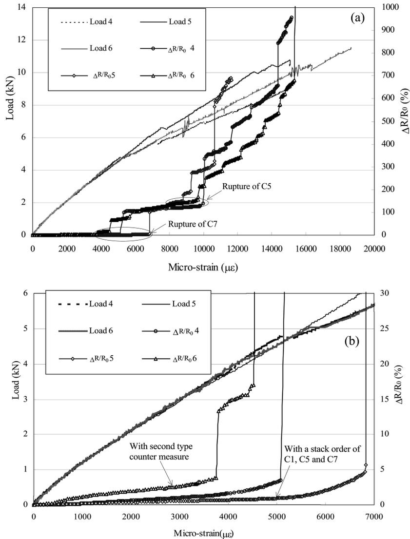
Fig. 9 Evolutions of load and  $\Delta R/R_0$  with micro-strain for specimens 4-6 with C1,C5 and C7 in a ration of 1:1:1 adhesively bonded on the surface of Dyneema sheet during whole strain range (a); during the low strain range (b).
