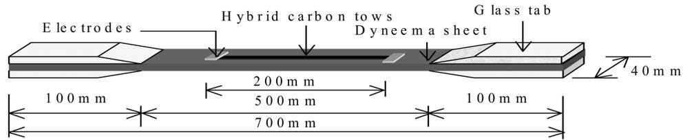
Fig. 1 Schematic dimension of the HCFRP sensor adhere on a layer of Dyneema sheet
