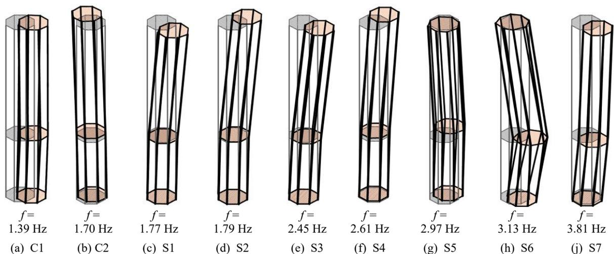
Fig. 7 Selected vibration modes of the Main Spire (SSI-Cov, June 6<sup>th</sup>, 2018, h 18:00-19:00)
