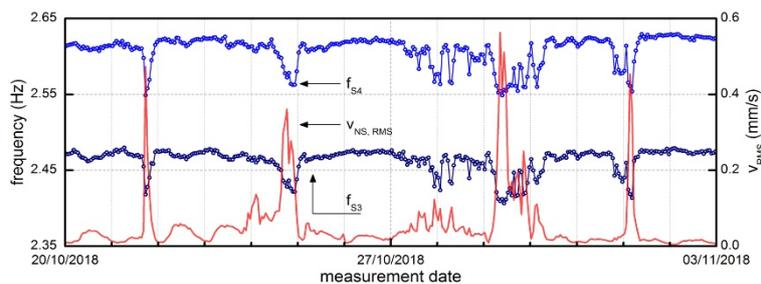
Fig. 13 Wind effects on frequencies  $f_{S3}$  and  $f_{S4}$
