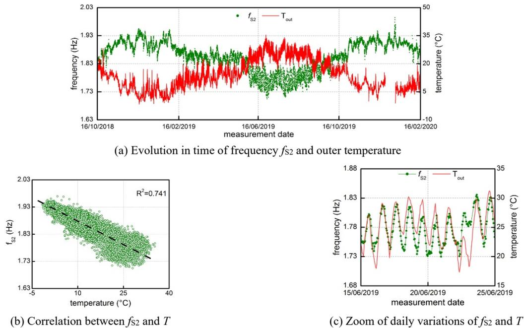
Fig. 11 Temperature effects on natural frequency  $f_{S2}$
