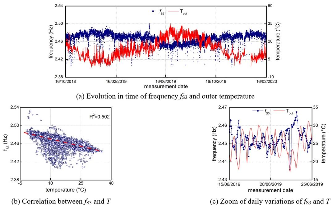
Fig. 12 Temperature effects on natural frequency  $f_{S3}$
