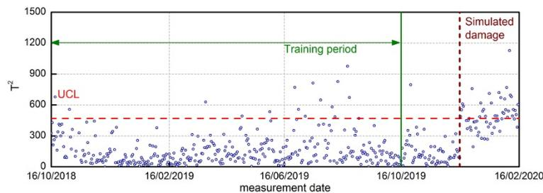
Fig. 17 Hotelling's  $T^2$  control chart obtained by simulating slight frequency shifts
