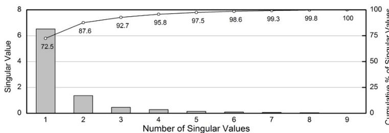
Fig. 14 Singular values of covariance matrix of natural frequencies (bars) and sum (lines)
