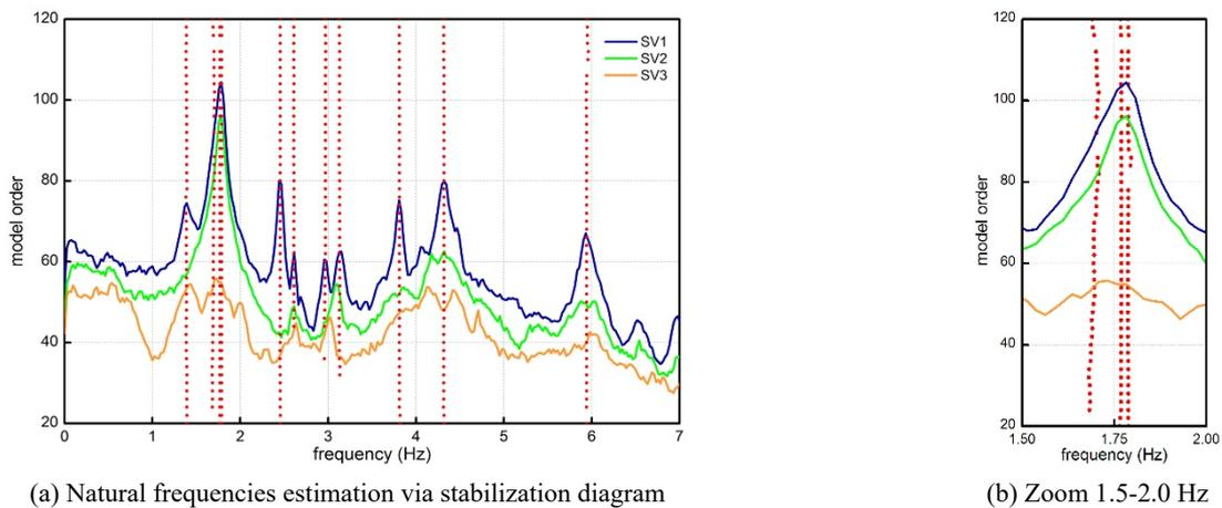
Fig. 6 Application of the SSI-Cov technique to signals collected in the Main Spire of Milan Cathedral (8 channels of velocity data, June 6<sup>th</sup>, 2018, h 18:00-19:00)
