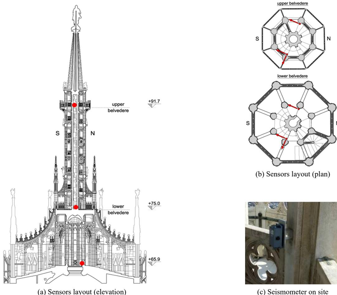
Fig. 4 Dynamic monitoring system installed in the Main Spire
