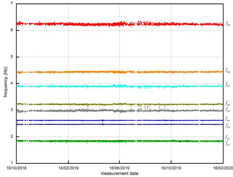
Fig. 15 Time evolution of the cleansed natural frequencies (4 principal components retained) from October 16th, 2018 to February 15th, 2020
