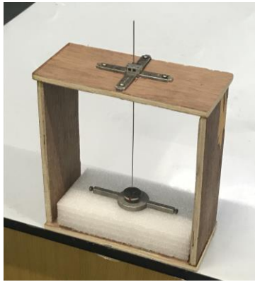
Fig. 5 The tiny TMD system used to experimentally identify its structural parameters
