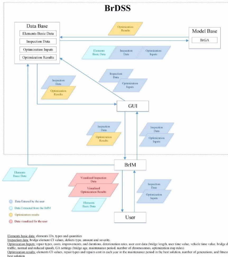
Fig. 1 BrDSS structure and its interaction with BrIM
