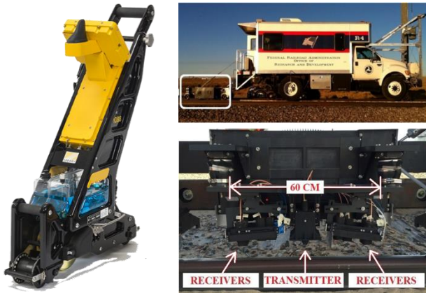
Fig. 1 Commercialized mobile ultrasonic inspection devices for detecting damage in railway tracks: (a) portable rail detector (Clark 2004); and (b) air-coupled ultrasound transducer-based detection vehicle (Mariani et al. 2017)
