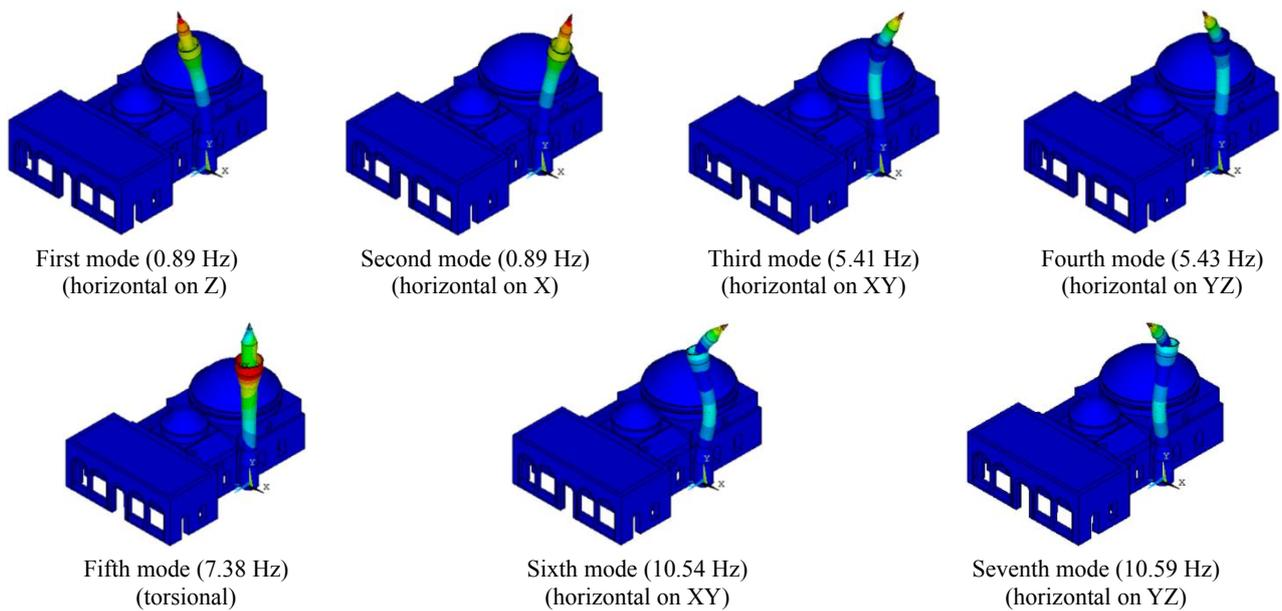
Fig. 11 First seven numerical mode shapes of the İskenderpaşa Mosque minaret
