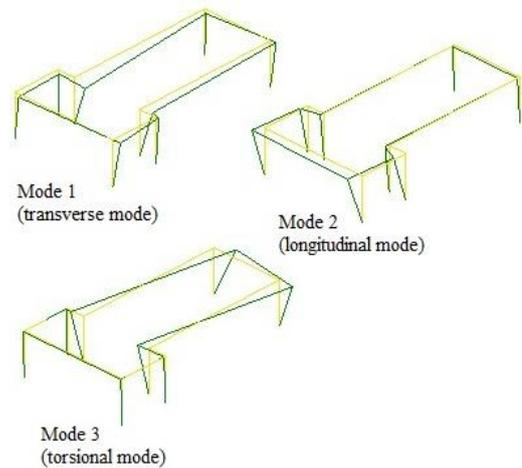
Fig. 8 The first three experimental modes of the mosque
