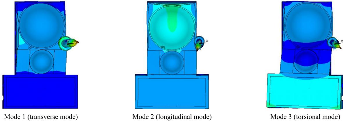
Fig. 10 The first three numerical modes of the mosque
