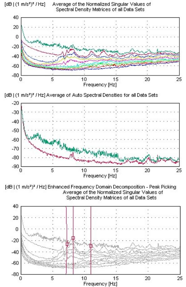
Fig. 6 ANSVSDM, AASD of the data sets, and selected picks from the SVSDM of the data sets obtained using EFDD method for the mosque
