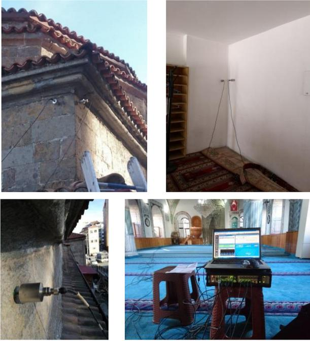
Fig. 4 The accelerometer connections and test equipment
