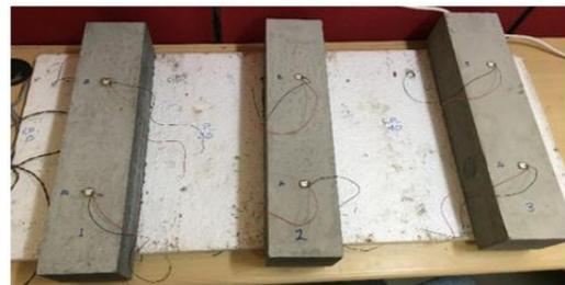
Fig. 2 Instrumentation using PZT for acquiring the impedance from cement composite specimens
