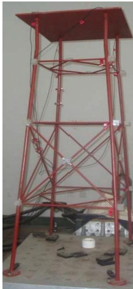
Fig. 8 The measured structure of offshore platform
