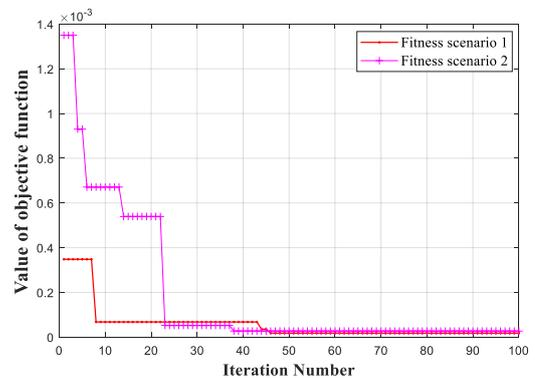
Fig. 16 Fitness of two damage scenarios (crack lengths 4 mm and 10 mm) using TLBO
