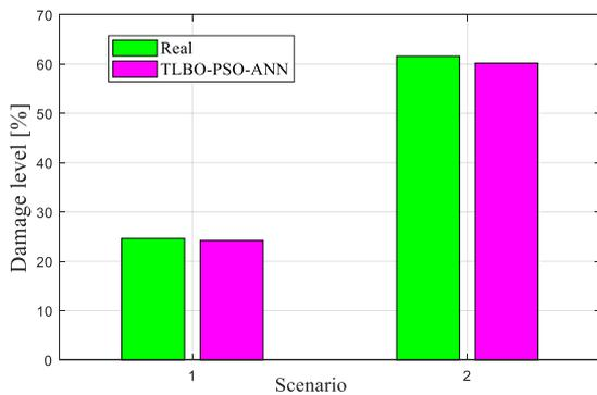
Fig. 15 Level of damage for crack lengths 4 mm and 10 mm calculated by TLBO-PSO-ANN
