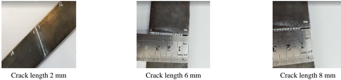
Fig. 13 Examples of crack configurations
