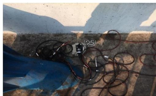
(b) Accelerometer (PCB-393B12)
