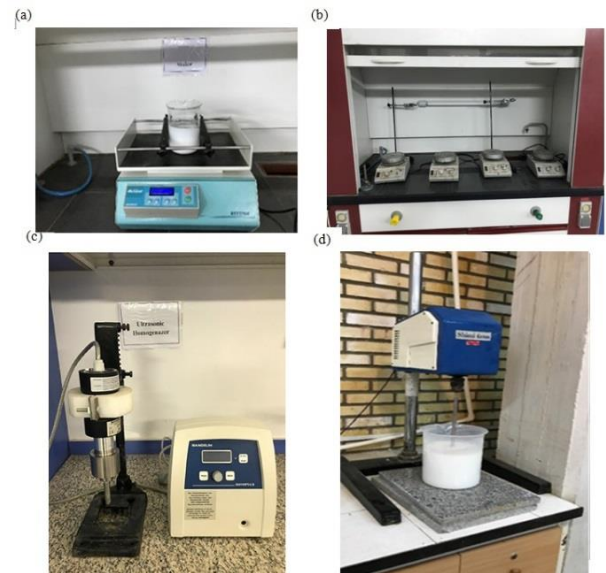
Fig. 1 The procedure of dispersing nano-capsules in the water (a) shaker; (b) magnetic stirrer; (c) ultrasonic devices (d) mechanical mixer
