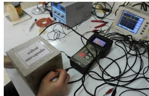
Fig. 4 The ultrasonic test for the cubic concrete samples
