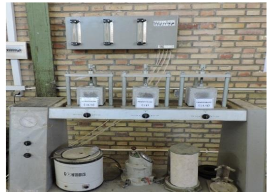
Fig. 9 The water penetration depth device
