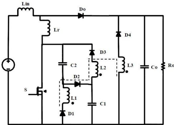
Fig. 1 The boost converter with proposed snubber
