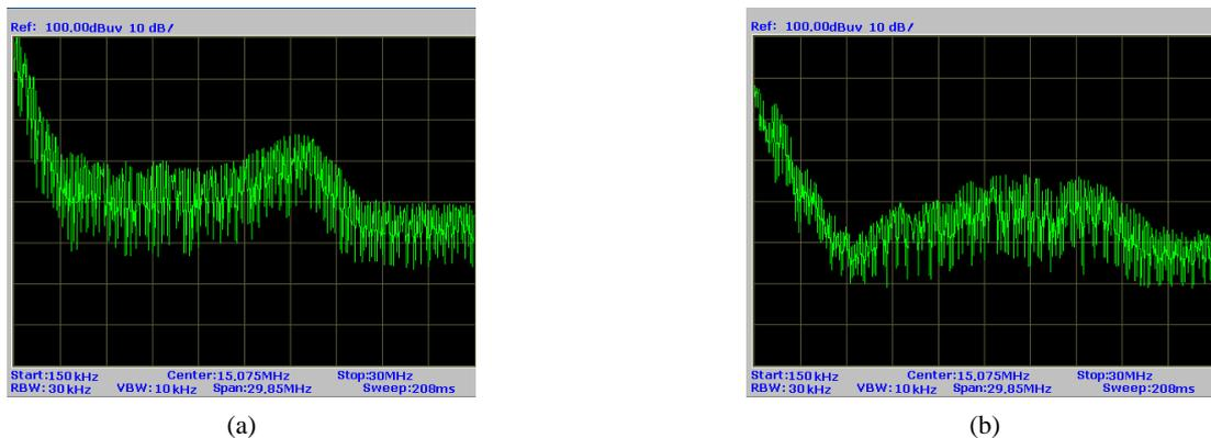
Fig. 16 Conducted EMI measurement. (a) hard-switching boost converter; (b) proposed boost converter; (Ver. axis: 20–100 dB $\mu$ V; Hor.axis: 0.15–30 MHz)
