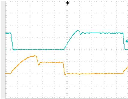
Fig. 10 Top: voltage wave form of converter switch (40 V/div); Bottom: current wave form of converter switch (2.5 A/div), (Time: 1  $\mu$ s/div)
