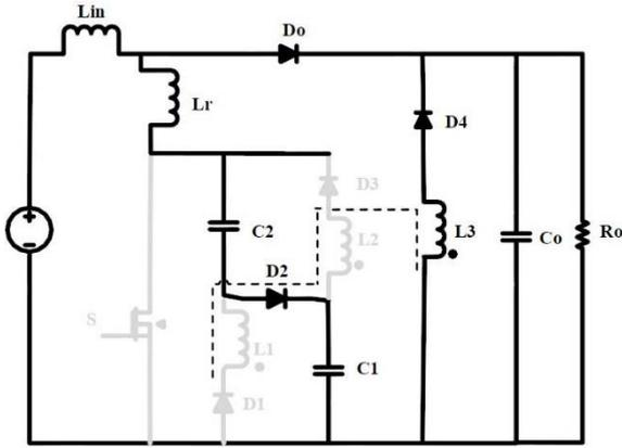
Fig. 8 The operation of the proposed circuit in the sixth Mode
