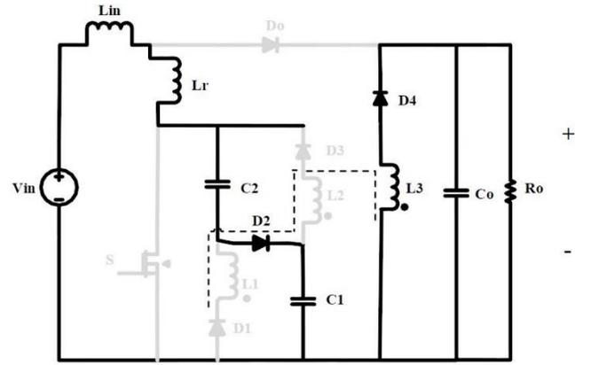
Fig. 7 The operation of the proposed circuit in the fifth Mode
