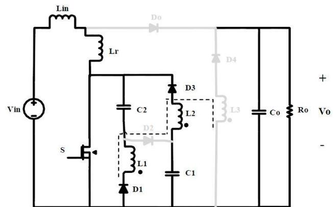
Fig. 4 The operation of the proposed circuit in the second Mode
