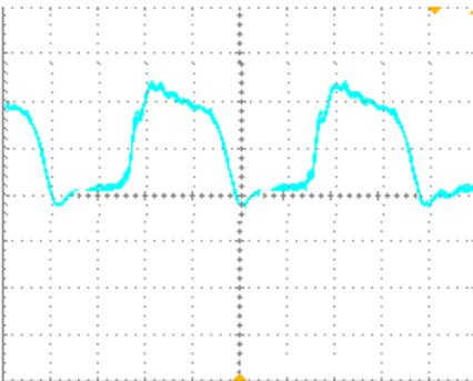
Fig. 11 Current wave form of diode D1 in the proposed boost converter (250 mA/div), (Time: 2.5  $\mu$ s/div)
