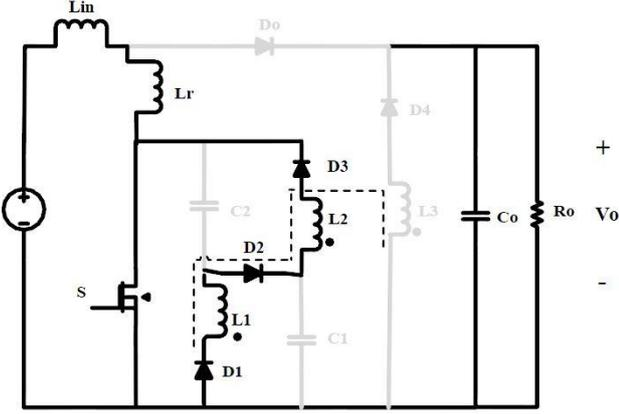
Fig. 5 The operation of the proposed circuit in the third Mode
