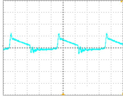
Fig. 14 Current waveform of diode D0 in proposed boost converter (5 A/div), (Time: 2.5  $\mu$ s/div)
