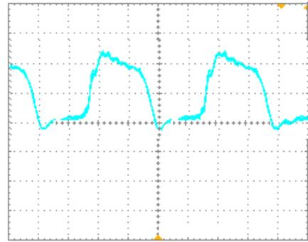
Fig. 13 Current waveform of diode D3 in proposed boost converter (250 mA/div), (Time: 2.5  $\mu$ s/div)
