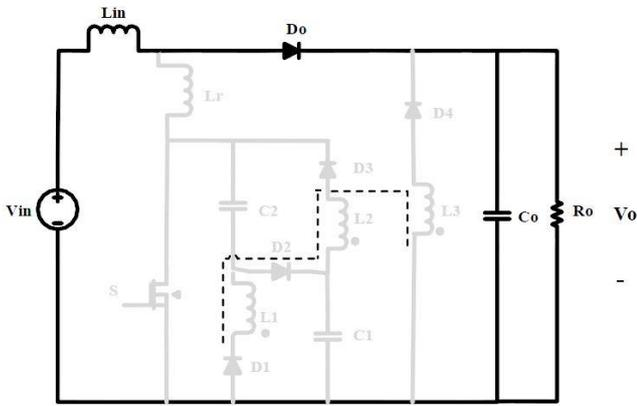
Fig. 9 The operation of the proposed circuit in the seventh Mode
