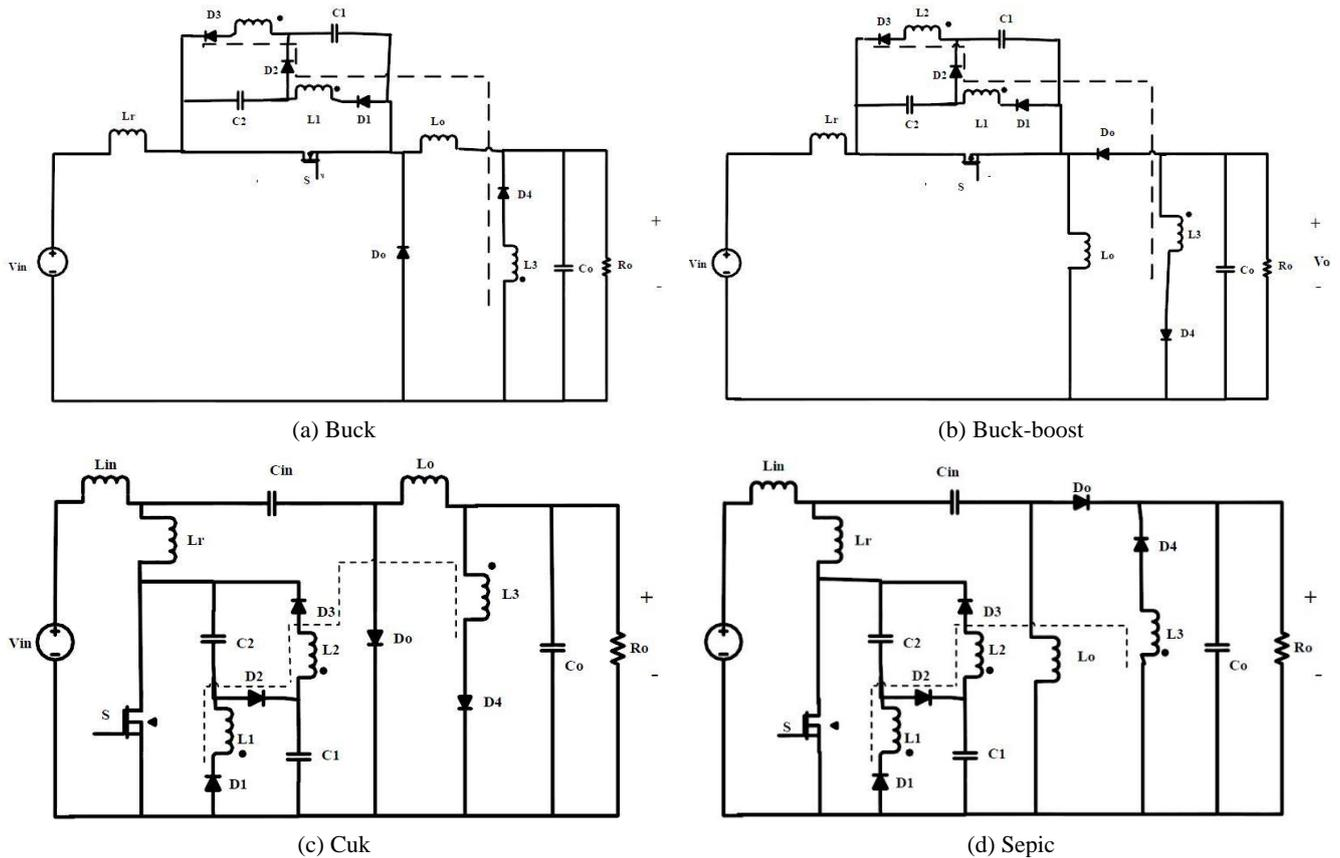
Fig. 15 The other soft switching converters with the proposed lossless snubber
