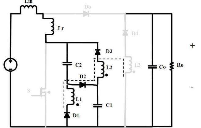
Fig. 6 The operation of the proposed circuit in the fourth Mode
