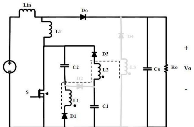
Fig. 3 The operation of the proposed circuit in the first Mode
