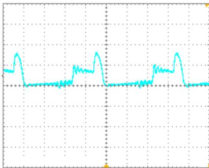
Fig. 12 Current wave form of diode D<sub>2</sub> in the proposed boost converter (1 A/div), (Time: 2.5  $\mu$ s/div)
